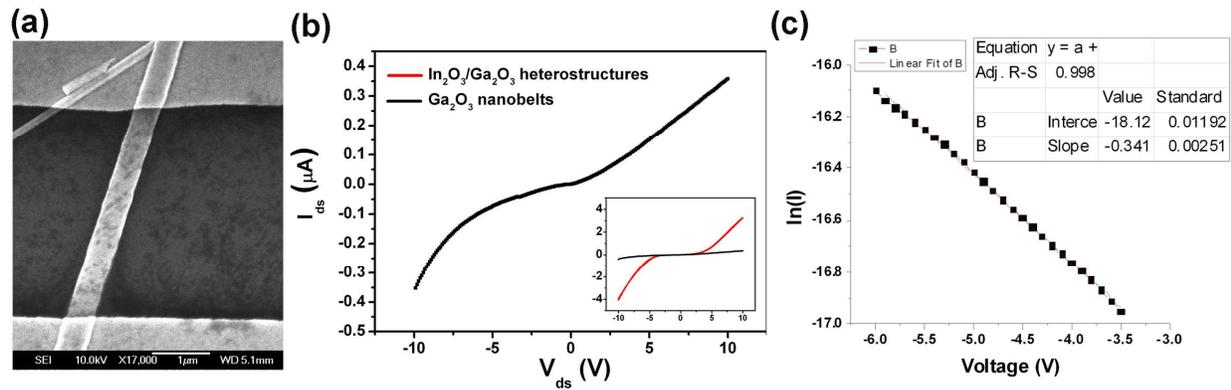
**Figure S3.** (a) SEM image of a Ga<sub>2</sub>O<sub>3</sub> nanobelt-based FET. (b)  $I_{ds}$ - $V_{ds}$  curves measured with  $V_g = 0 \text{ V}$ . (c) Experimental and fitted  $\ln I$  vs  $V$  plots at an intermediate bias using the  $I$ - $V$  curve in (b).
