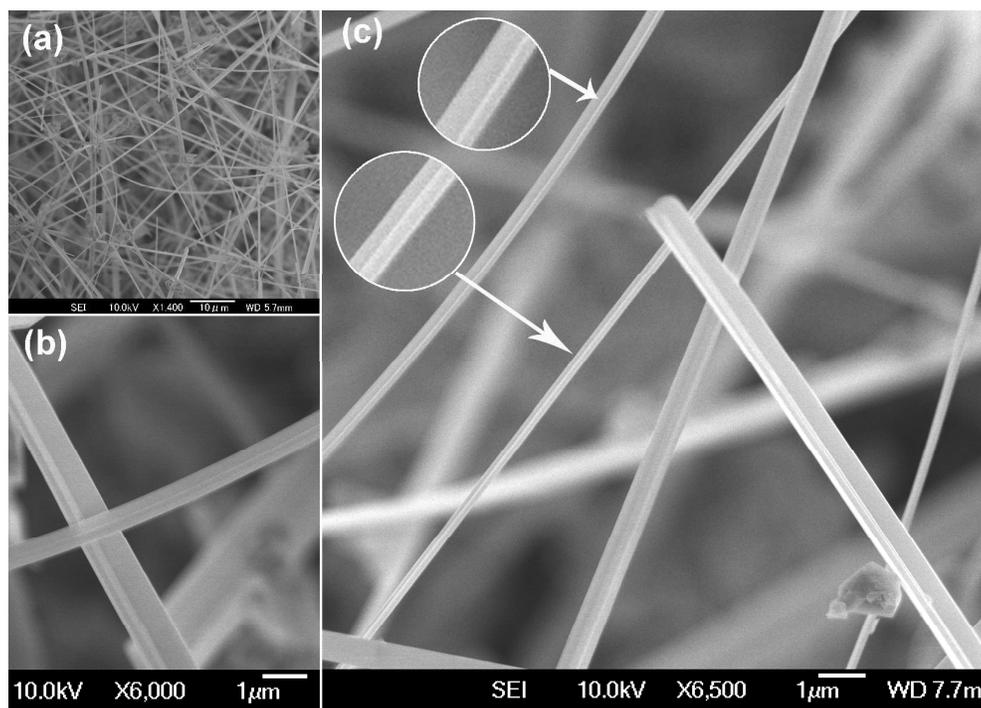
**Figure S1.** (a) Low- and (b,c) high-magnification SEM images reveal that the product consists of numerous 1D heterostructures .
