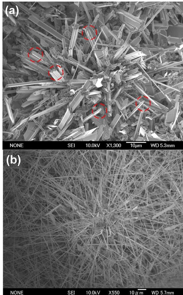
**Figure S2.** SEM images of products synthesized over different reaction times. (a) After reaction for 10 min. The image clearly shows many 1D heterostructures with short lengths grow on the copper foil substrate, indicating that the heteroepitaxial growth of heterostructures occurred at very early stages of the reaction process. (b) After reaction for 1 h. The final product consists of numerous heterostructures with high aspect ratio.
