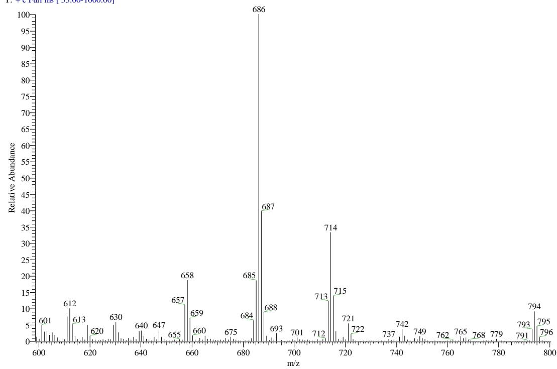
**Figure S9.** Pyrolysis mass spectrum of TDPB at 270-450 °C,  $m/z$  = 600-800.
