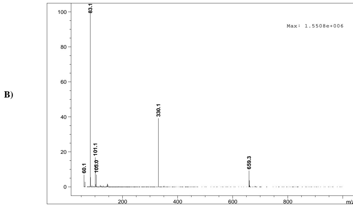
**Figure S10.** Isolated DPBP product A) HPLC trace 50-100% MeCN gradient for 30 min, 1mL/min, mass spectral detector, and B) corresponding mass spectrum.
