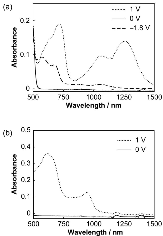
**Figure S3.** UV–vis–NIR spectra of compounds **1** (a) and **2** (b) in  $\text{CH}_2\text{Cl}_2$  solutions (1.0 mM) observed under the application of the oxidation and reduction potentials using a Pt mesh working electrode. The supporting electrolyte is  $\text{Bu}_4\text{NClO}_4$  (0.10 M).
