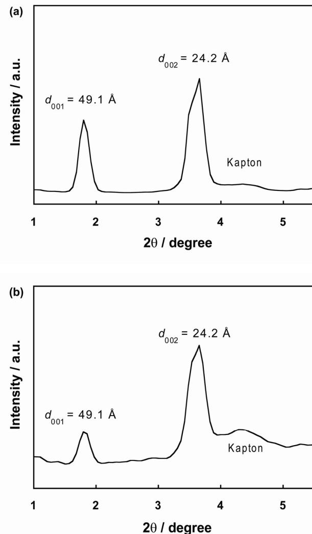
**Figure S5.** Small-angle X-ray scattering patterns for **1** at 160 °C (a) and for **2** at 120 °C (b). The shoulders at 4.4 degrees in the small-angle X-ray scattering patterns are attributed to the Kapton film placed between the sample and the X-ray detector.
