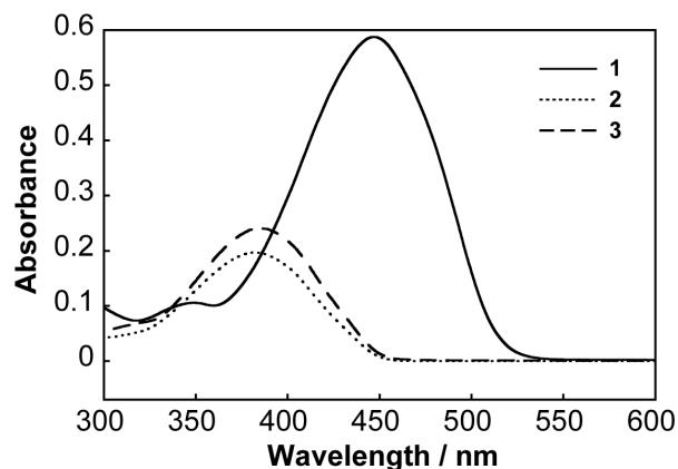
**Figure S2.** Absorption spectra for **1–3** in chloroform solutions ( $1 \times 10^{-7}\text{ M}$ ).
