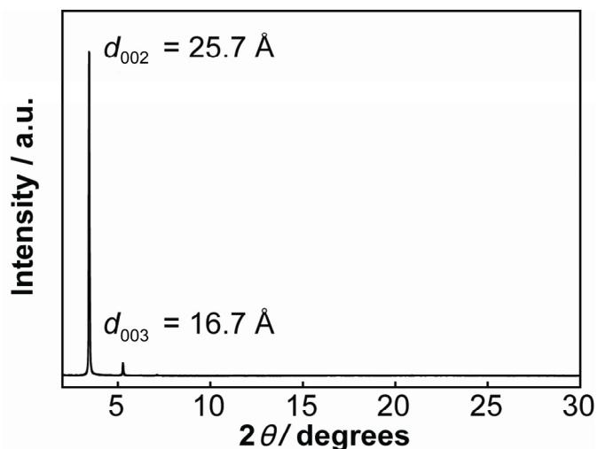
**Figure S4.** X-ray diffraction pattern for **2** in the SmA phase at 120 °C.
