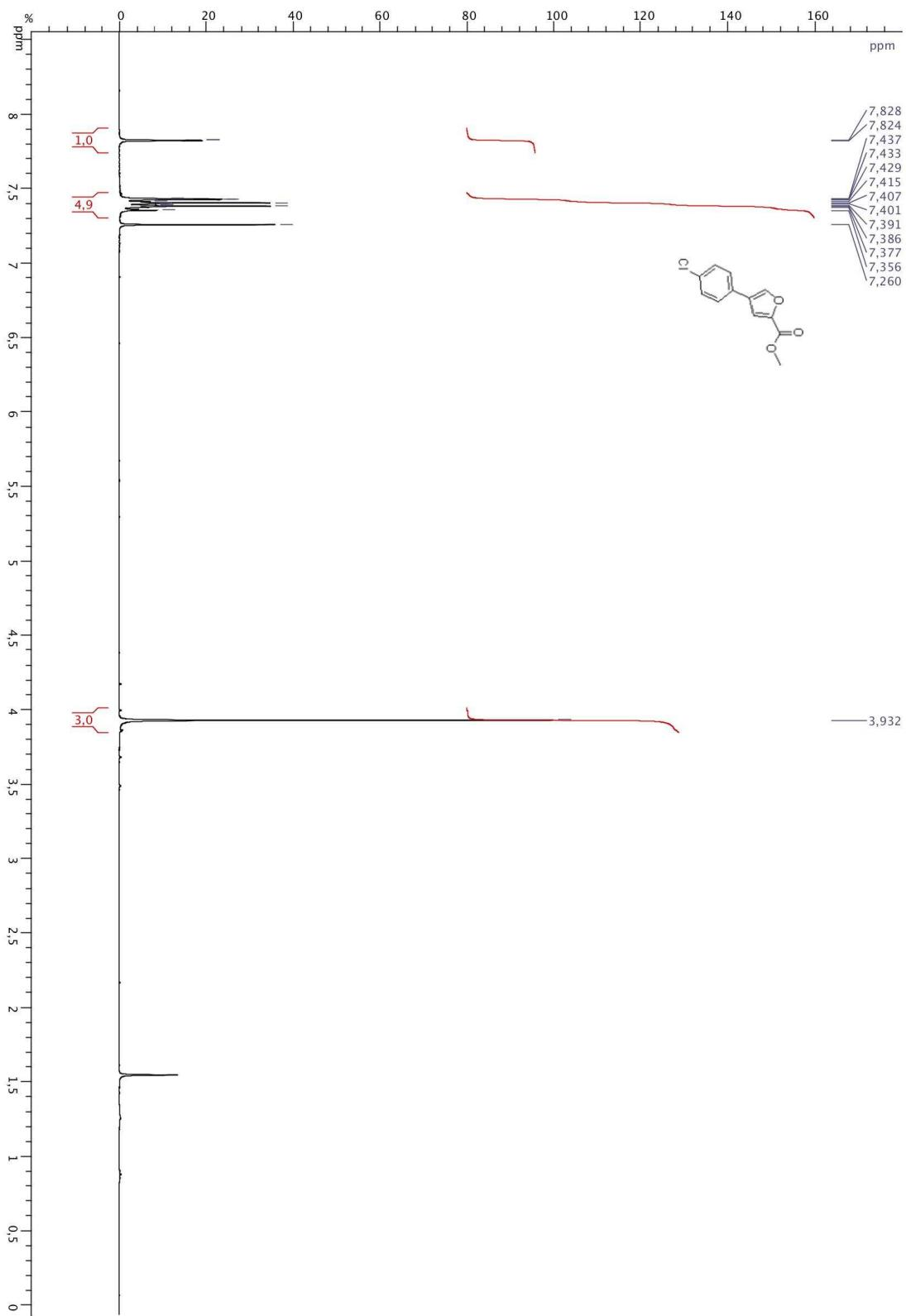
**<sup>13</sup>C NMR of methyl 4-(4-chlorophenyl)furan-2-carboxylate (CDCl<sub>3</sub>, 75 MHz)**
