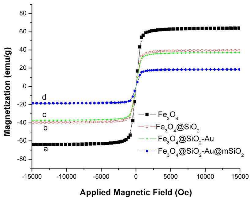
**Figure S3.** The magnetic hysteresis loops of (a) the  $\text{Fe}_3\text{O}_4$  particles, (b) the core-shell  $\text{Fe}_3\text{O}_4@SiO_2$  microspheres, (c) the  $\text{Fe}_3\text{O}_4@SiO_2\text{-Au}$  microspheres and (d) the  $\text{Fe}_3\text{O}_4@SiO_2\text{-Au@mSiO}_2$  microspheres with 90-nm thickness outer mesoporous silica layer.
