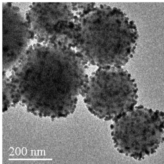
**Figure S2.** The TEM image of the  $\text{Fe}_3\text{O}_4@ \text{SiO}_2\text{-Au}$  microspheres with a low magnification, showing that the  $\text{Fe}_3\text{O}_4@ \text{SiO}_2$  microspheres were evenly decorated with Au nanoparticles of about 12 nm in size.
