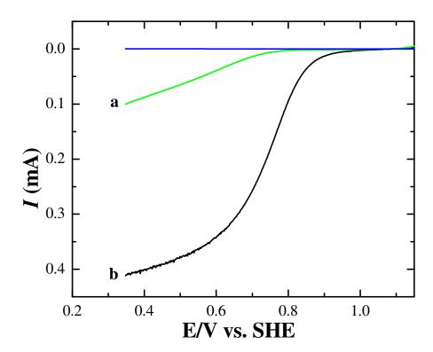
Figure 8S  $Tafel\ plot\ obtained\ for\ ORR\ in\ 0.5\ M\ H_2SO_4\ on\ nPtF\ modified\ electrode.$
