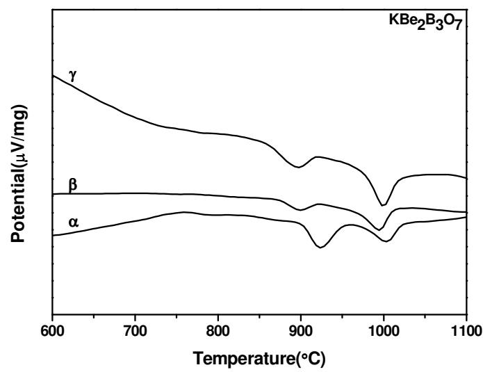
b. DTA trace for the compositions of  $\text{KBe}_2\text{B}_3\text{O}_7$
