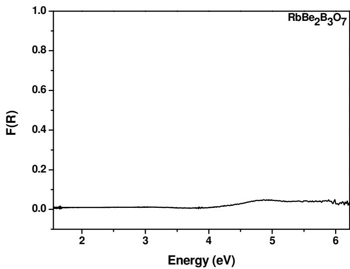
d. Diffuse reflectance absorption curve of the powder sample of  $\text{RbBe}_2\text{B}_3\text{O}_7$
