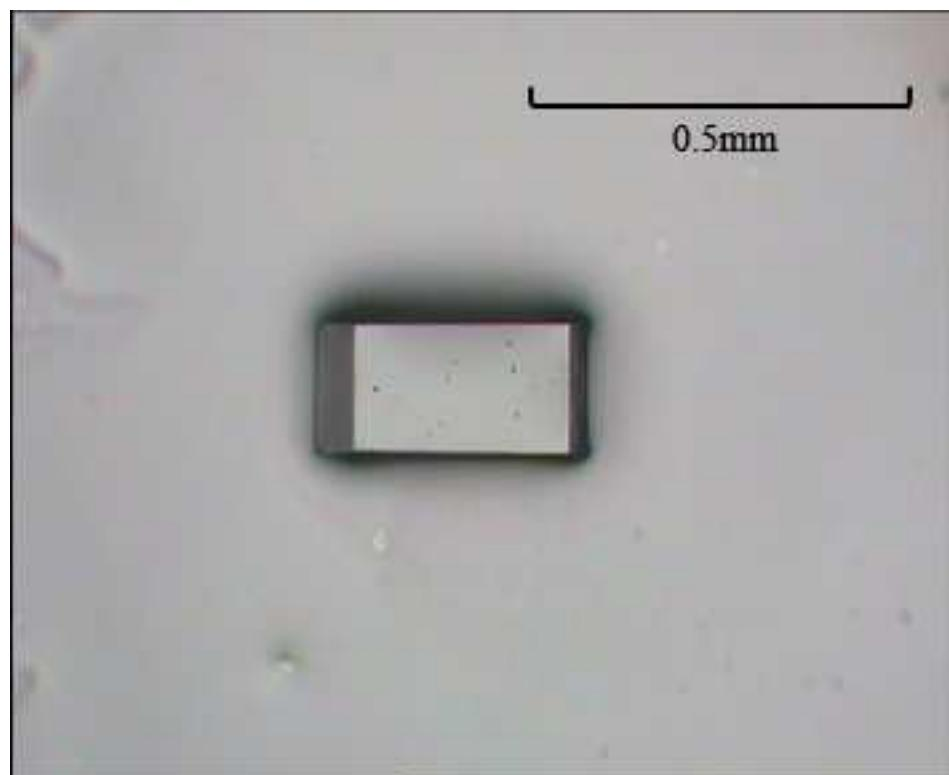
d. As-grown  $\gamma$ -KBe<sub>2</sub>B<sub>3</sub>O<sub>7</sub> crystal
