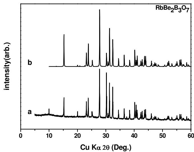
e. X-ray powder diffraction patterns of  $\text{RbBe}_2\text{B}_3\text{O}_7$
