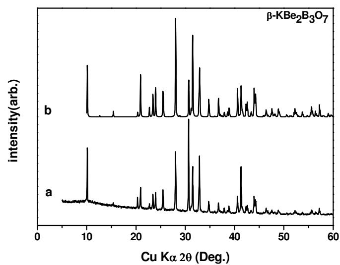
c. X-ray powder diffraction patterns of  $\beta$ -KBe<sub>2</sub>B<sub>3</sub>O<sub>7</sub>
