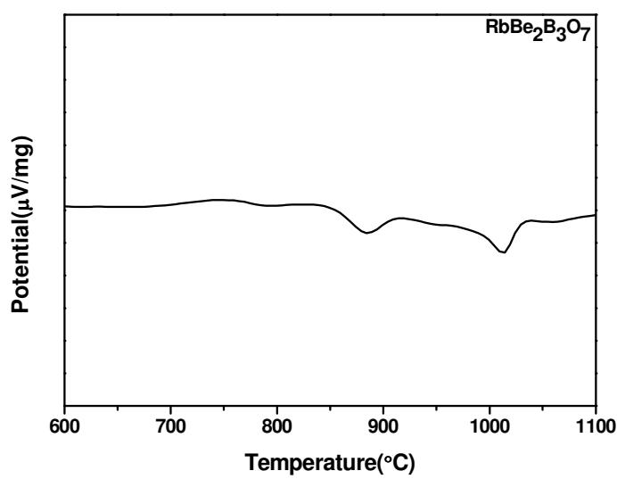
c. DTA trace for the compositions of  $\text{RbBe}_2\text{B}_3\text{O}_7$
