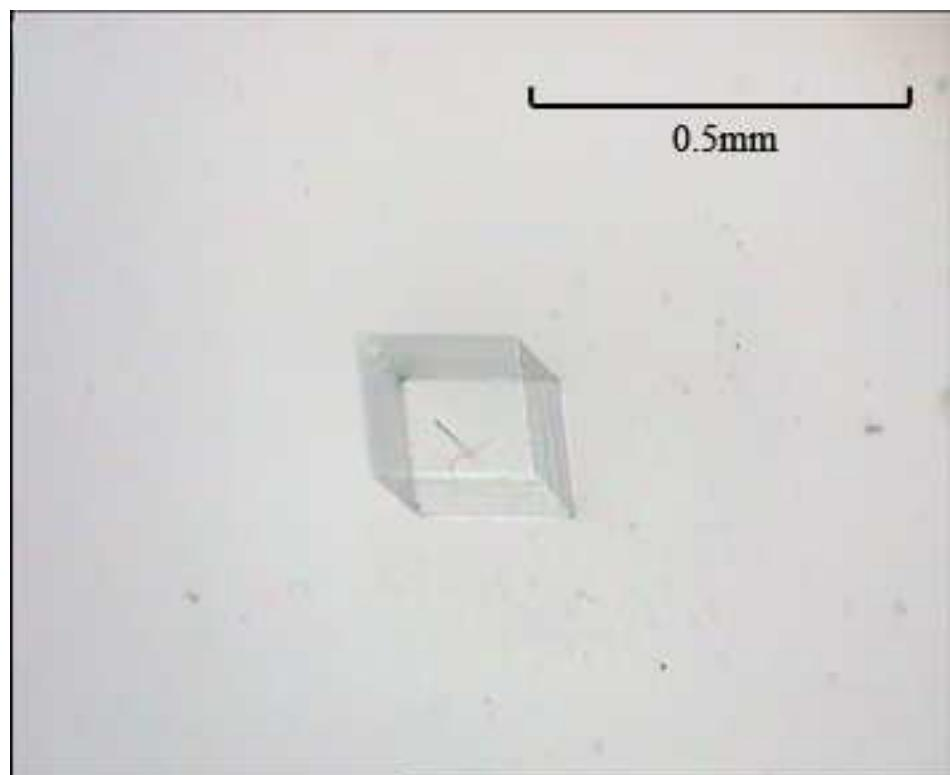
b. As-grown  $\alpha$ -KBe<sub>2</sub>B<sub>3</sub>O<sub>7</sub> crystal
