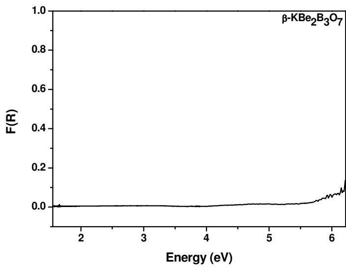
b. Diffuse reflectance absorption curve of the powder sample of  $\beta$ -KBe<sub>2</sub>B<sub>3</sub>O<sub>7</sub>
