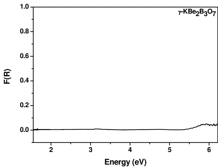
c. Diffuse reflectance absorption curve of the powder sample of  $\gamma$ -KBe<sub>2</sub>B<sub>3</sub>O<sub>7</sub>
