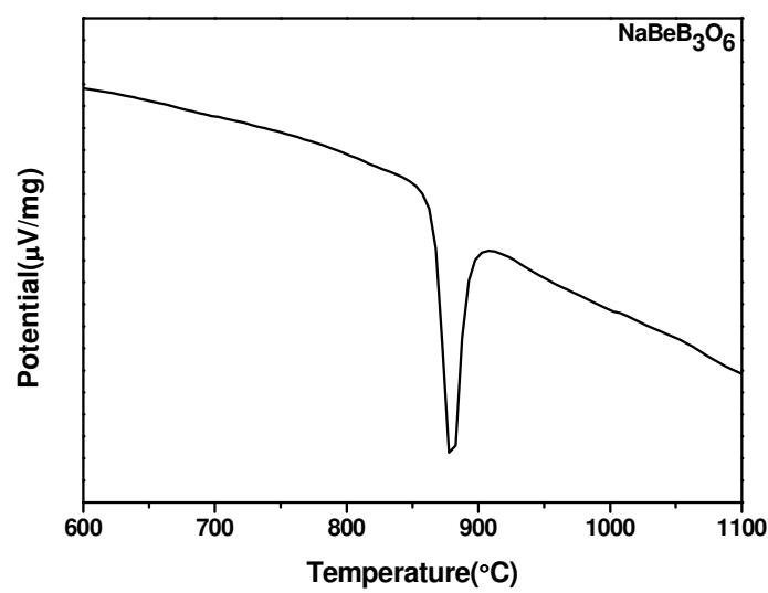
a. DTA trace for the compositions of  $\text{NaBeB}_3\text{O}_6$
