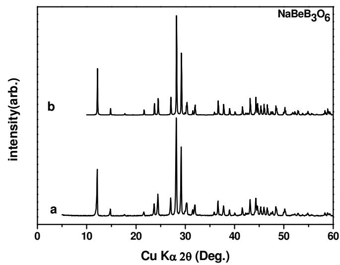
a. X-ray powder diffraction patterns of  $\text{NaBeB}_3\text{O}_6$
