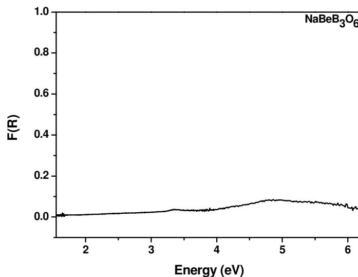
a. Diffuse reflectance absorption curve of the powder sample of  $\text{NaBeB}_3\text{O}_6$
