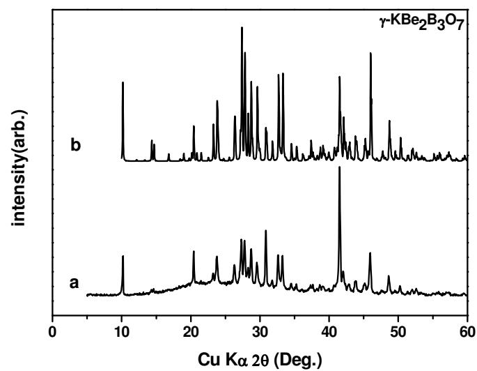
d. X-ray powder diffraction patterns of  $\gamma$ -KBe<sub>2</sub>B<sub>3</sub>O<sub>7</sub>
