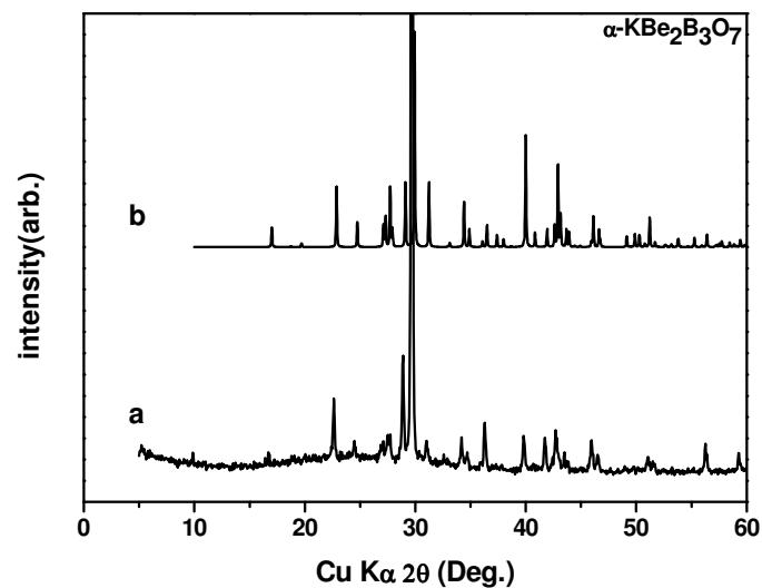
b. X-ray powder diffraction patterns of  $\alpha\text{-KBe}_2\text{B}_3\text{O}_7$
