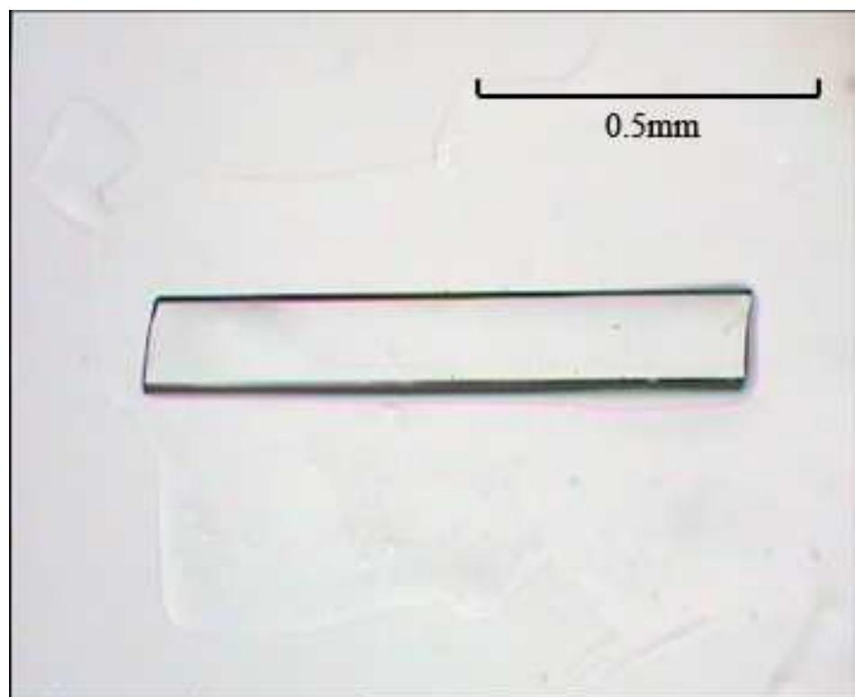
c. As-grown  $\beta$ -KBe<sub>2</sub>B<sub>3</sub>O<sub>7</sub> crystal
