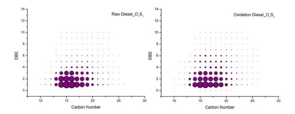
Figure S-1. Plots of double bond equivalents (DBE) as a function of carbon number for the  $O_1S_1$  class derived from the positive-ion ESI FT-ICR mass spectrum of the raw and oxidized diesel samples (Figure 3).
