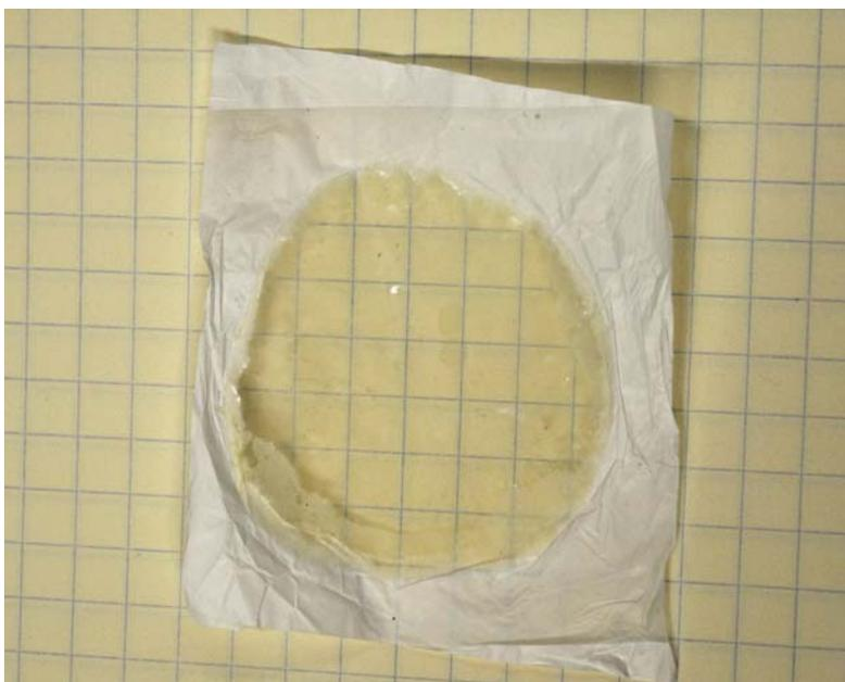
**Figure S9.** Picture of a supported cross-linked Q<sub>I</sub>-phase membrane of **2c**. Scale: Each grid division is 0.25 of an inch. The polymerized Q<sub>I</sub>-phase of **2c** infused into the Solupor support is visually transparent, while the surrounding pristine Solupor support material is not.
