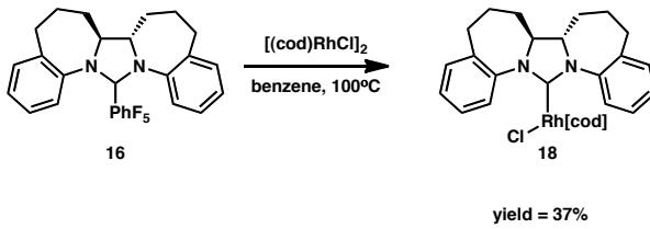
In the glovebox, a 25 mL Schlenck flask equipped with a stirbar was charged with [Rh(COD)Cl]<sub>2</sub> (18 mg, 0.073 mmols) and the pentafluorophenyl adduct (34 mg, 0.072 mmols). To this was added 2 mL of benzene. The flask was sealed, removed from the glovebox and heated at 100°C for 48h. The reaction mixture was purified on silica gel (50% ether/hexanes) to afford a crystalline yellow solid. A single rotational isomer was identified in solution.
