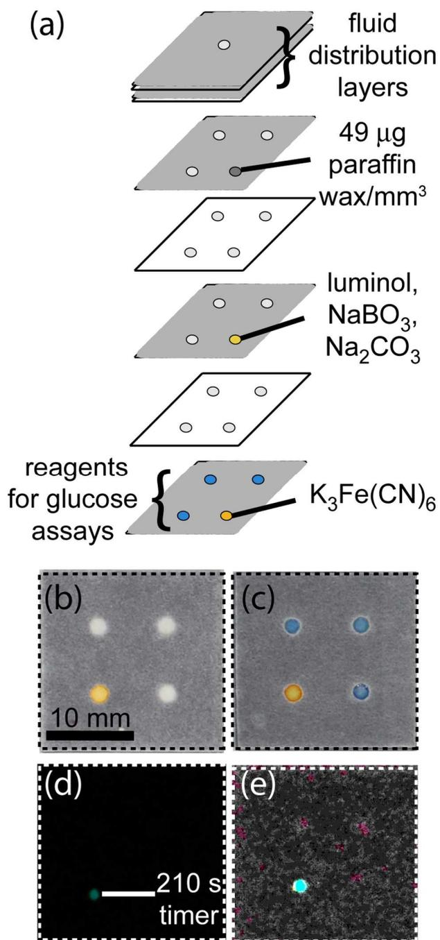
**Figure S11.** A 3D  $\mu$ PAD containing a fluidic timer that provides a chemiluminescent signal when the assay is complete. (a) Expanded view of the layers of the 3D  $\mu$ PAD. The  $\mu$ PAD has one 210 s fluidic timer, and three conduits for measuring the level of glucose in the sample. (b) Photograph of the bottom of the 3D  $\mu$ PAD prior to applying sample to the device. The
