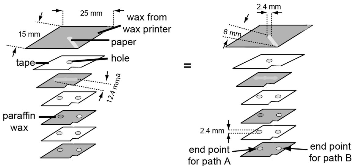
**Figure S4.** Dimensions of the device described in Figure 4.
