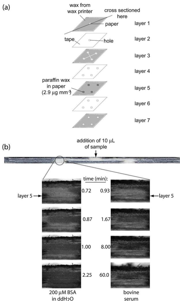
**Figure S8.** Effect of the type of fluids on the fluid distribution rates through a 3D  $\mu\text{PAD}$  that contains a meter. (a) Expanded top view of the device with a dotted line that indicates where the device was cut in half. (b) Black and white time-lapsed photographs showing the cross-
