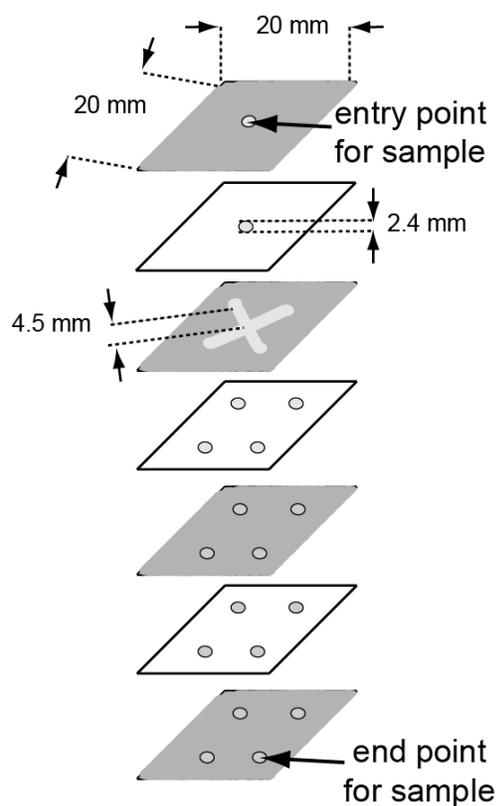
**Figure S1.** Dimensions of the device described in Figure 1. The length of the 4.5-mm channel in the image begins at the bottom of the circular end region of the channel and extends to the center of the point where the channels cross. The devices shown in Figures 5 and S10–12 possess nearly identical dimensions, with the exception that the number of layers is different in each device.
