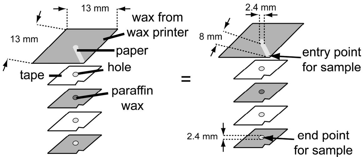
**Figure S5.** Dimensions of the devices used in Table 2.
