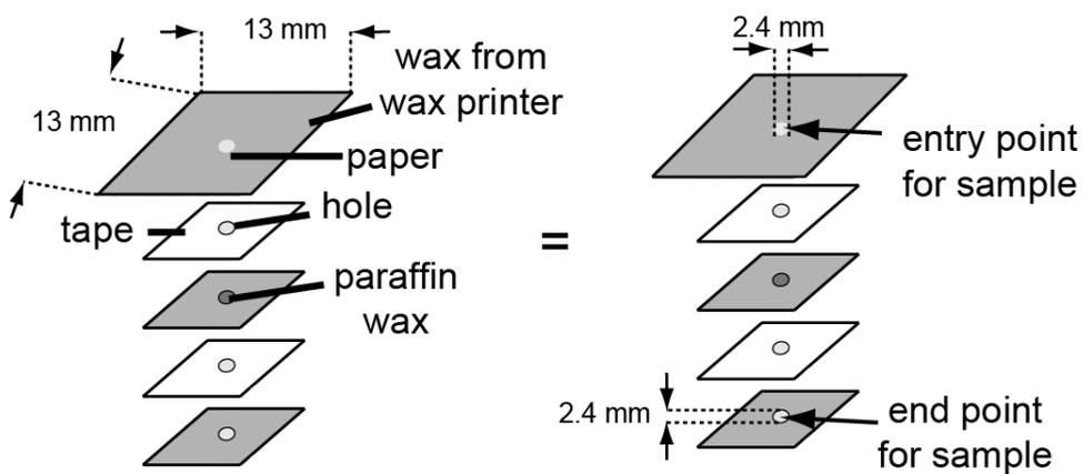
**Figure S3.** Dimensions of the device described in Figure 3.
