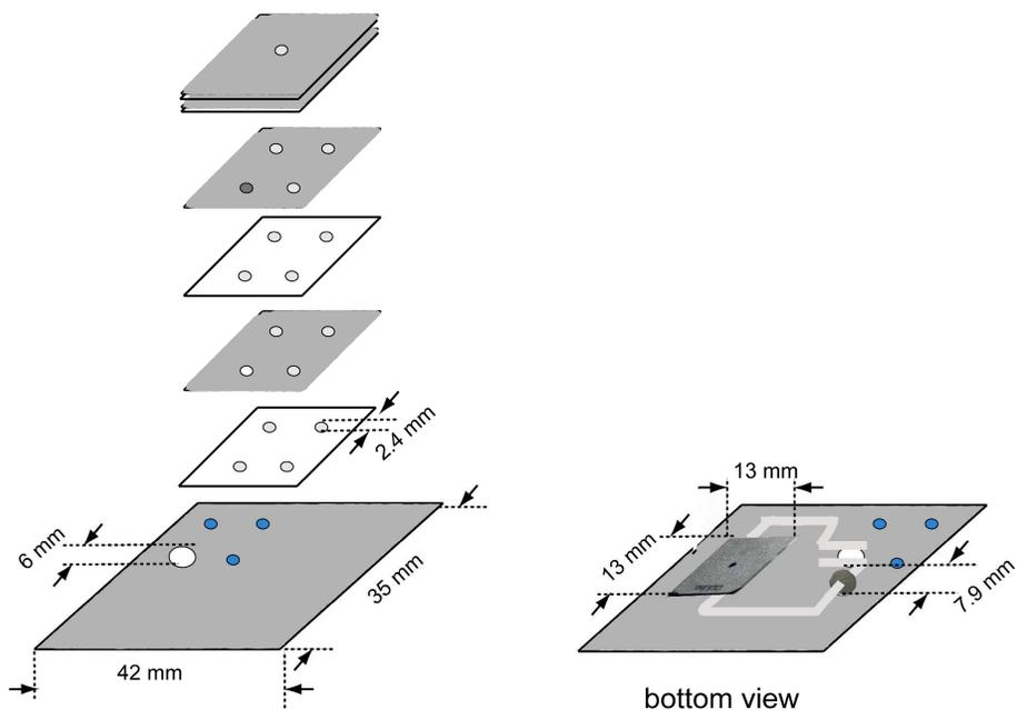
**Figure S6.** Dimensions of the device described in Figure S12.
