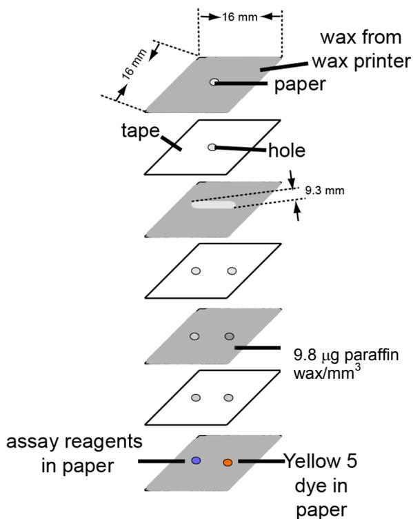
**Figure S2.** Dimensions of the device described in Figure 2.
