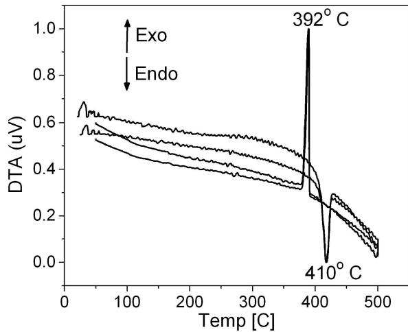
**Figure S7.** DTA of  $\text{K}_6\text{As}_2(\text{P}_2\text{Se}_6)_3$ . The pure compound melts congruently at  $410^\circ\text{C}$  and recrystallizes at  $392^\circ\text{C}$  with no significant shifts observed upon running multiple cycles.
