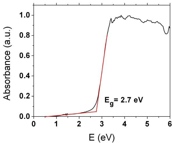
**Figure S21.** Diffuse reflectance UV-Vis spectrum of  $\text{Cs}_5\text{As}(\text{P}_2\text{S}_6)_2$ . The estimated band gap of 2.7eV matches well with the yellow color of the crystals.
