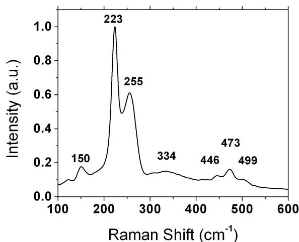
**Figure S18.** Raman spectrum of  $\text{Cs}_5\text{As}(\text{P}_2\text{Se}_6)_2$ . The strongest peak at  $223\text{ cm}^{-1}$  is indicative of the  $A_{1g}$  stretch of  $[\text{P}_2\text{Se}_6]^{4-}$ . All others are also consistent with the anion.
