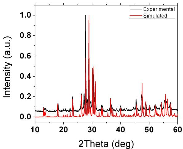
**Figure S10.** Experimental (black) and simulated (red) PXRD of  $\text{Cs}_6\text{As}_2(\text{P}_2\text{Se}_6)_3$ . All peaks match between the two patterns indicating a pure compound.
