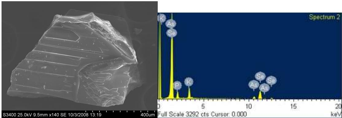
**Figure S1.** SEM micrograph and corresponding EDS spectrum of a K<sub>7</sub>As<sub>3</sub>(P<sub>2</sub>Se<sub>6</sub>)<sub>4</sub> crystal. The average composition of multiple scans was K<sub>6.2</sub>As<sub>3.0</sub>P<sub>9.4</sub>Se<sub>24.7</sub>.
