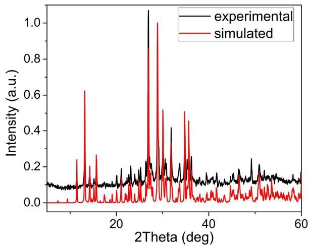
**Figure S5.** Experimental (black) and simulated (red) PXRD of  $\text{K}_6\text{As}_2(\text{P}_2\text{Se}_6)_3$ . All peaks match between the two patterns indicating a pure compound.
