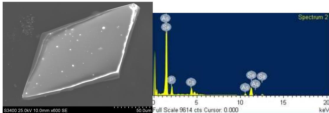
**Figure S9.** SEM micrograph and corresponding EDS spectrum of a  $\text{Cs}_6\text{As}_2(\text{P}_2\text{Se}_6)_3$  crystal. The average composition of multiple scans was  $\text{Cs}_{6.1}\text{As}_{2.0}\text{P}_{6.7}\text{Se}_{18.3}$ .
