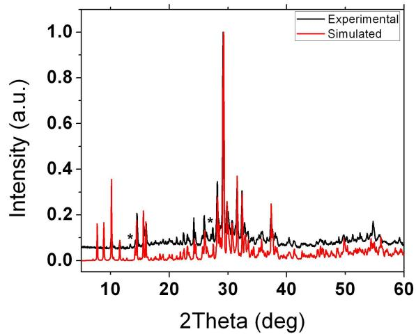
**Figure S2.** Experimental (black) and simulated (red) PXRD of K<sub>7</sub>As<sub>3</sub>(P<sub>2</sub>Se<sub>6</sub>)<sub>4</sub>. Minor impurity peaks are denoted with an asterisk (\*).
