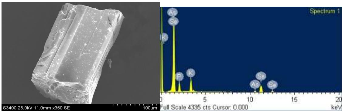
**Figure S4.** SEM micrograph and corresponding EDS spectrum of a  $\text{K}_6\text{As}_2(\text{P}_2\text{Se}_6)_3$  crystal. The average composition of multiple scans was  $\text{K}_{6.0}\text{As}_{2.0}\text{P}_{7.8}\text{Se}_{20.5}$ .
