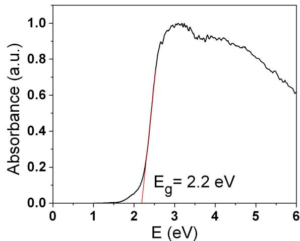
**Figure S6.** Diffuse reflectance spectrum of  $\text{K}_6\text{As}_2(\text{P}_2\text{Se}_6)_3$ . The sharp band gap transition at 2.2eV matches well with the orange color of the crystals.
