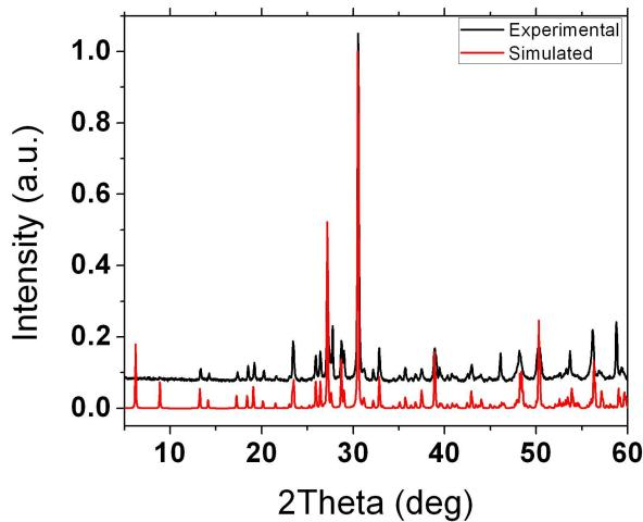
**Figure S15.** Experimental (black) and simulated (red) PXRD of  $\text{Cs}_5\text{As}(\text{P}_2\text{Se}_6)_2$ . All peaks match between the two patterns.
