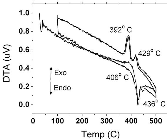
**Figure S20.** DTA of  $\text{Cs}_5\text{As}(\text{P}_2\text{S}_6)_2$ . The impurity,  $\text{Cs}_4\text{P}_2\text{S}_{10}$ , is reported to melt congruently at  $\sim 420^\circ\text{C}$ , indicating the consistent melting and recrystallization of **4b** at  $406^\circ\text{C}$  and  $392^\circ\text{C}$ , respectively.
