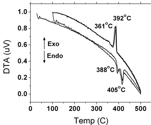
**Figure S3.** DTA of K<sub>7</sub>As<sub>3</sub>(P<sub>2</sub>Se<sub>6</sub>)<sub>4</sub>. Melting and crystallization of the major product, 1, are 388°C and 361°C, respectively, although the presence of the impurity is seen.
