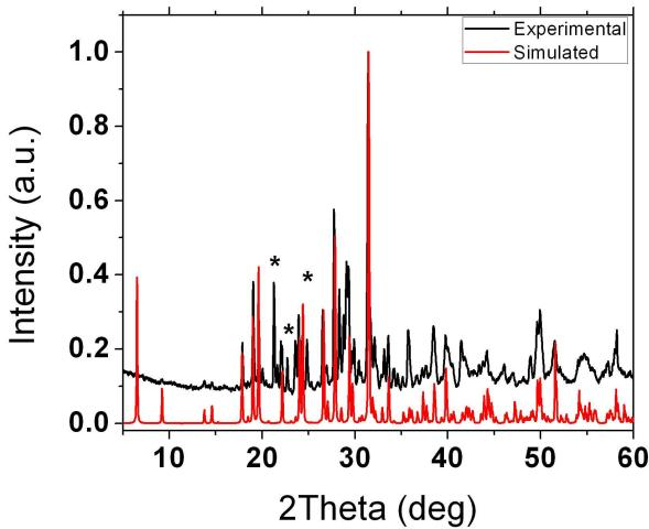
**Figure S19.** Experimental (black) and simulated (red) PXRD of  $\text{Cs}_5\text{As}(\text{P}_2\text{S}_6)_2$ . Impurity peaks are denoted with an asterisk (\*).
