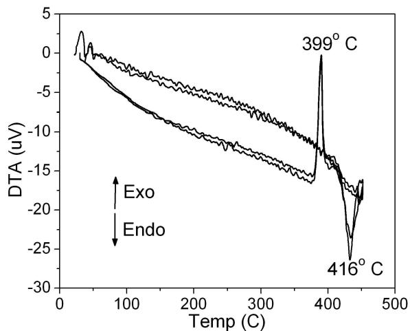
**Figure S16.** DTA of  $\text{Cs}_5\text{As}(\text{P}_2\text{Se}_6)_2$ . The pure compound melts congruently at  $416^\circ\text{C}$  and recrystallizes at  $399^\circ\text{C}$ .
