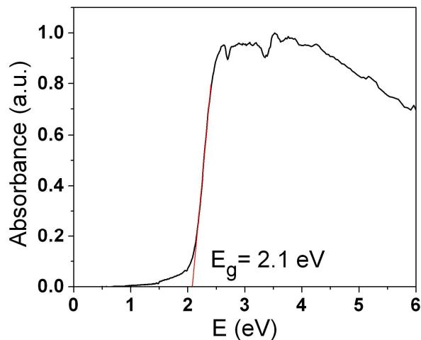
**Figure S12.** Diffuse reflectance UV-Vis spectrum of  $\text{Cs}_6\text{As}_2(\text{P}_2\text{Se}_6)_3$ . The estimated band gap of 2.1eV matches well with the orange color of the crystals.
