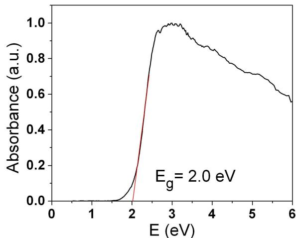
**Figure S17.** Diffuse reflectance UV-Vis spectrum of  $\text{Cs}_5\text{As}(\text{P}_2\text{Se}_6)_2$ . The estimated band gap of  $2.0\text{eV}$  matches well with the red color of the crystals.
