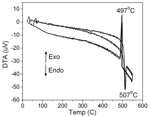
**Figure S11.** DTA of  $\text{Cs}_6\text{As}_2(\text{P}_2\text{Se}_6)_3$ . The pure compound melts congruently at 507°C and crystallizes at 497°C with no significant shifts observed upon running multiple cycles.
