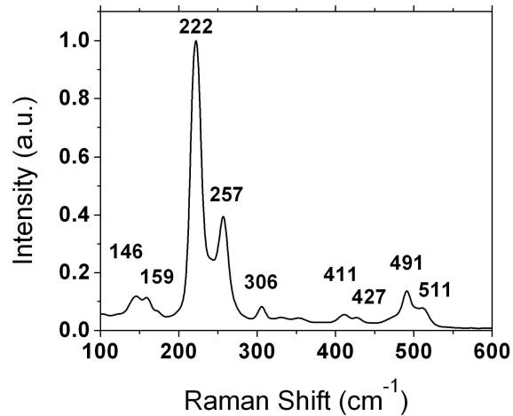
**Figure S8.** Raman spectrum of  $\text{K}_6\text{As}_2(\text{P}_2\text{Se}_6)_3$ . The strongest peak at  $222 \text{ cm}^{-1}$  can be assigned to the  $A_{1g}$  stretch of  $[\text{P}_2\text{Se}_6]^{4-}$ . All others are consistent with the anion as well.
