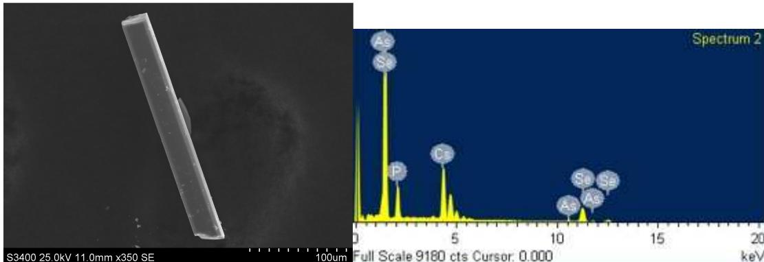
**Figure S14.** SEM micrograph and corresponding EDS spectrum of a  $\text{Cs}_5\text{As}(\text{P}_2\text{Se}_6)_2$  crystal. The average composition of multiple scans was  $\text{Cs}_{4.3}\text{As}_{1.0}\text{P}_{4.1}\text{Se}_{11.1}$ .
