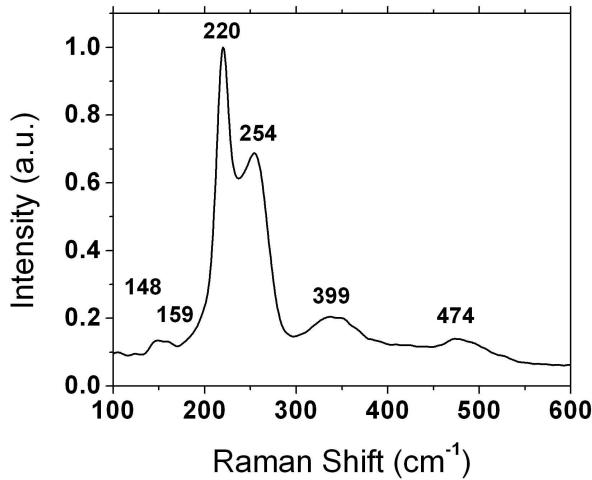
**Figure S13.** Raman spectrum of  $\text{Cs}_6\text{As}_2(\text{P}_2\text{Se}_6)_3$ . The strongest peak at  $220 \text{ cm}^{-1}$  is indicative of the totally symmetric stretch of  $[\text{P}_2\text{Se}_6]^{4-}$ . All others are also consistent with the anion.
