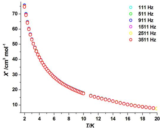
**Figure S6.** Frequency-dependent behavior of  $\chi'$  for **1** in zero static field.
