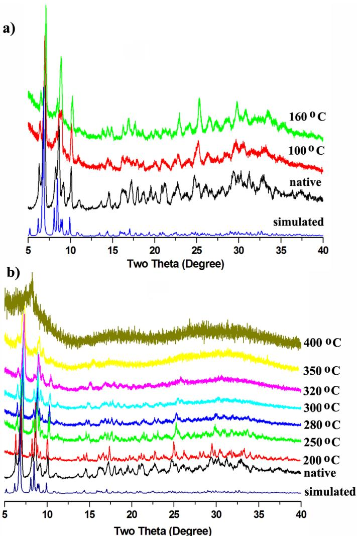
**Figure S3.** a) Hydrothermal stability of the as-synthesized sample **1**. b) Thermodiffractograms of the as-synthesized sample **1**.
