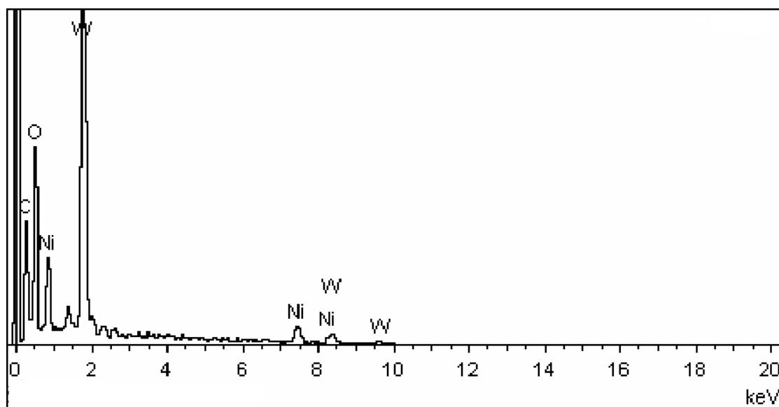
**Figure S9.** Energy-dispersive X-ray spectroscopy of **1**, showing there is no sodium in the structure.
