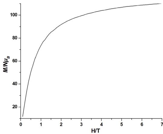
**Figure S7.** Magnetization measurement, in the reduced form of  $M/N\mu_B$ , in the field range 0 - 7 T at 2 K of **1**.
