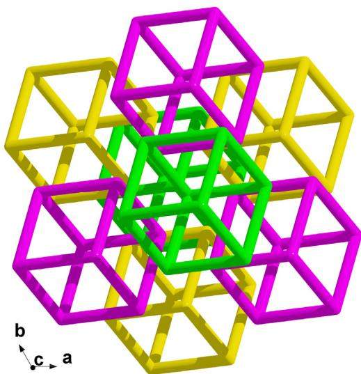
**Figure S2.** View of the 3D hexagonal close-packed structure of **1** along the *c*-axis. Tris-grafted  $Ni_6PW_9$  and the 1,3,5-BTCs are simplified as 3-connected nodes and linear bars respectively.
