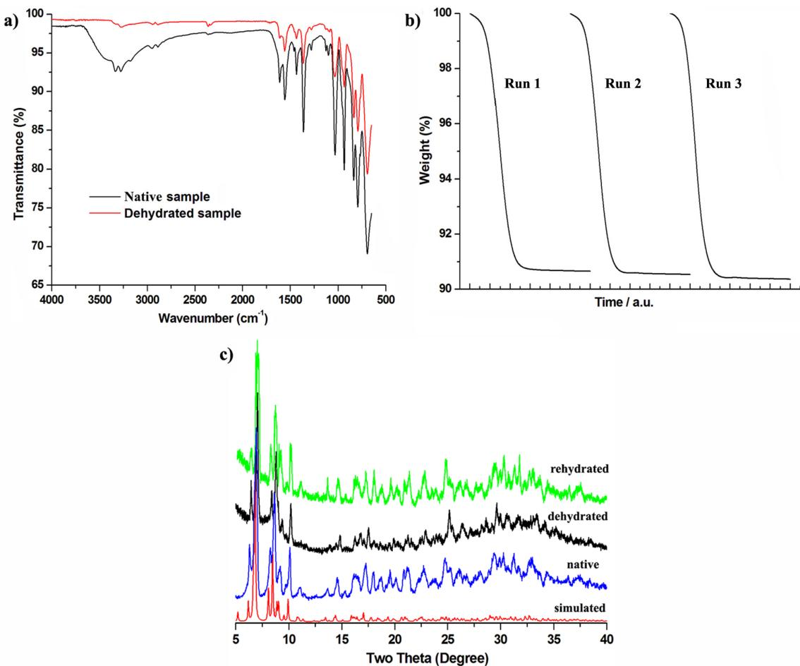
**Figure S8.** a) IR spectra of **1** before and after heated at 200 °C for one hour. b) TGA water desorption of **1** showing three consecutive runs. c) PXRD patterns of **1** as simulated from single crystal XRD, native sample, after dehydration and after rehydration (room temperatures).
