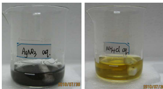
Figure S18. The cationic exchange experiments of 1 in 1 \text{ mol} \cdot \text{L}^{-1} \text{ AgNO}_3 (left) and 1 \text{ mol} \cdot \text{L}^{-1} \text{ NH}_4\text{Cl} aqueous solution (right).
