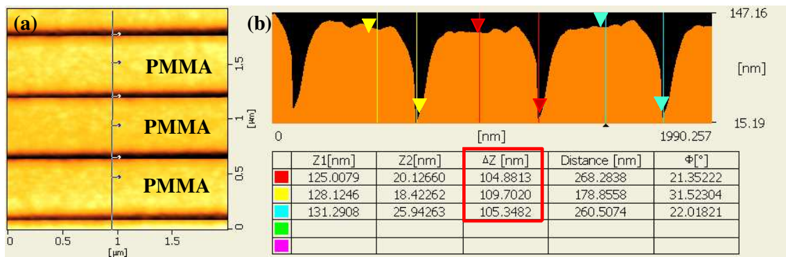
Figure S1. AFM image for PMMA patterned using electron beam lithography process: (a) image of the patterned PMMA; (b) scan profile along the line in image (a).
