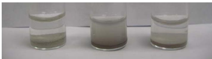
**Fig. S1.** Tollens mirror reaction of (left) (PLL/PLGA)<sub>3.5</sub>-, (middle) (PLL/PLGA)<sub>3.5</sub>-GA-, and (right) (PLL/PLGA)<sub>3.5</sub>-GA-PLL-shelled particles. Excessive PLL was used to react with the aldehyde groups of GA in the last step in forming (PLL/PLGA)<sub>3.5</sub>-GA-PLL-shelled particles. As a result, no aldehyde groups remain in (PLL/PLGA)<sub>3.5</sub>-GA-PLL-shelled particles.
