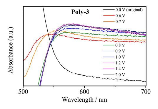
**Figure S1.** Differential UV-vis spectra of **Poly-3** film cast on an ITO glass electrode. Obtained at various applied potentials (vs.  $Ag^+/Ag$ ). The UV-vis spectrum of the original **Poly-3** film is also shown.
