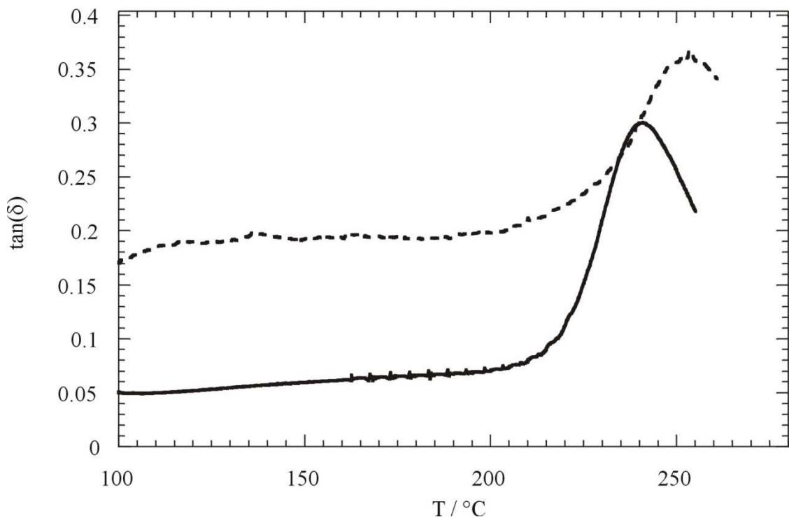
Fig. 5s. The loss tangent as a function of temperature for HM pectin/HNTs. —  $C_f = 20\%$ , ---  $C_f = 60\%$ .
