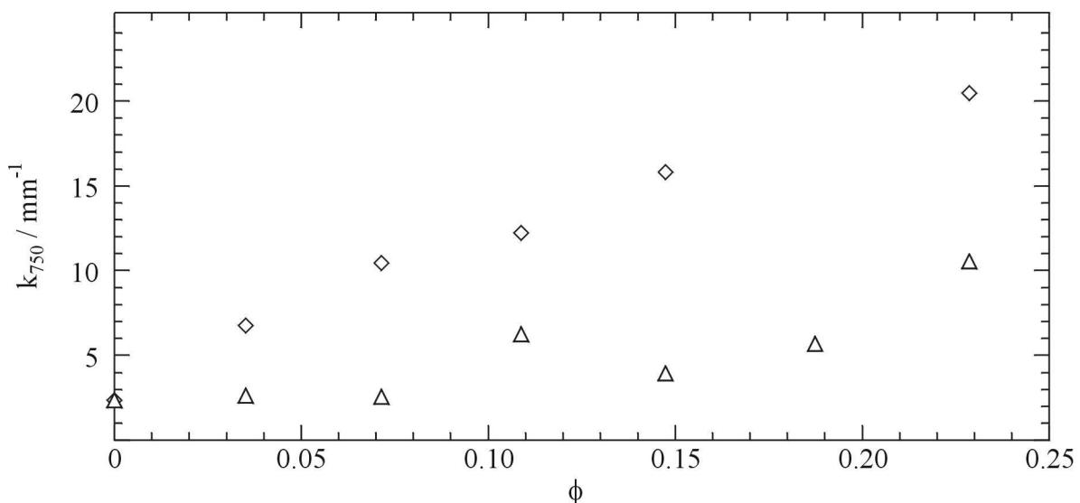
Figure 11s. Dependence of the attenuation coefficient at 750 nm on the filler volume fraction for LM Pectin mixed with HNTs ( $\diamond$ ) and laponite RD ( $\Delta$ ).
