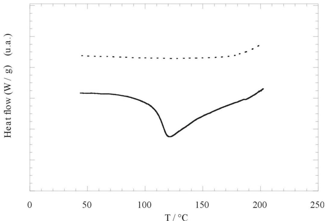
Figure 10s. Thermogram of LM Pectin. Full line is during heating and dotted line is upon cooling.
