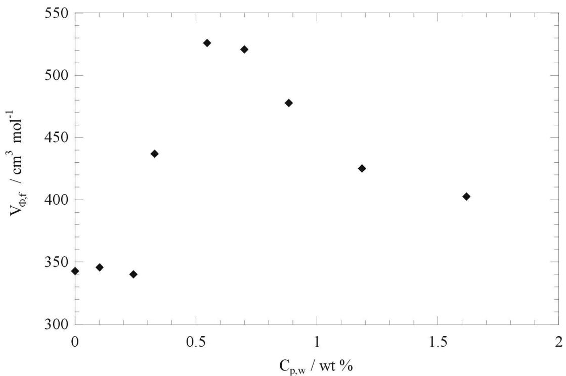
Figure 12s. Apparent molar volume of laponite RD as a function of LM pectin concentration at 35 °C. The error is within the symbols being  $\pm 0.4 \text{ cm}^3 \text{mol}^{-1}$ .
