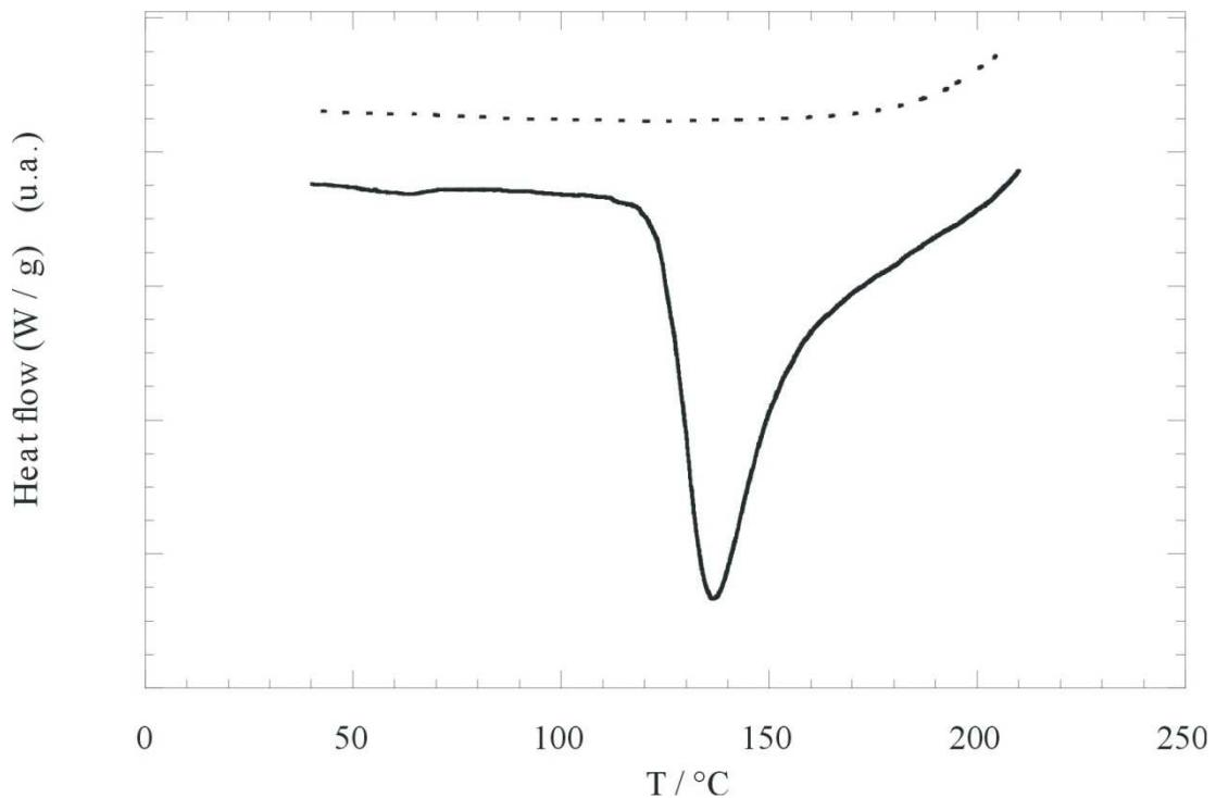
Figure 9s. Thermogram of HM Pectin. Full line is during heating and dotted line is upon cooling.
