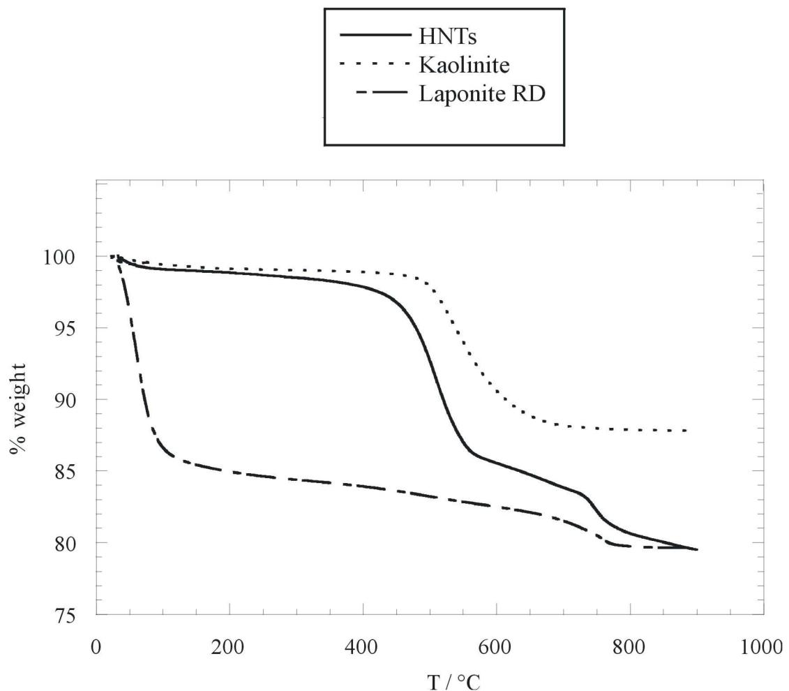
Fig. 8s TG curves of the used nanofillers
