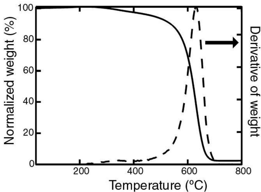
**Figure S4. Thermogravimetric analysis of the as-prepared composite via heating at a rate of 2°C/min under dry air flow showed only one peak suggesting a monolithic chemical composition.**
