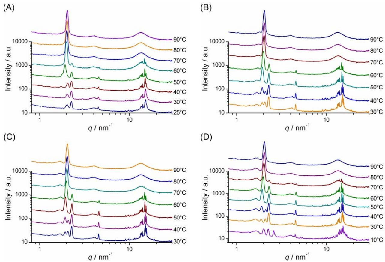
**Figure 9.** Small- and wide-angle X-ray scattering curves of neat ChC16 at various temperatures and heating-cooling cycles: (A) freshly heated, (B) first cooling, (C) re-heated and (D) second cooling.
