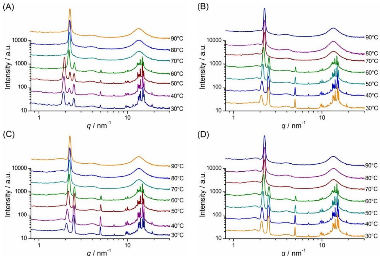
**Figure 8.** Small- and wide-angle X-ray scattering curves of neat ChC14 at various temperatures and heating-cooling cycles: (A) freshly heated, (B) first cooling, (C) re-heated and (D) second cooling.
