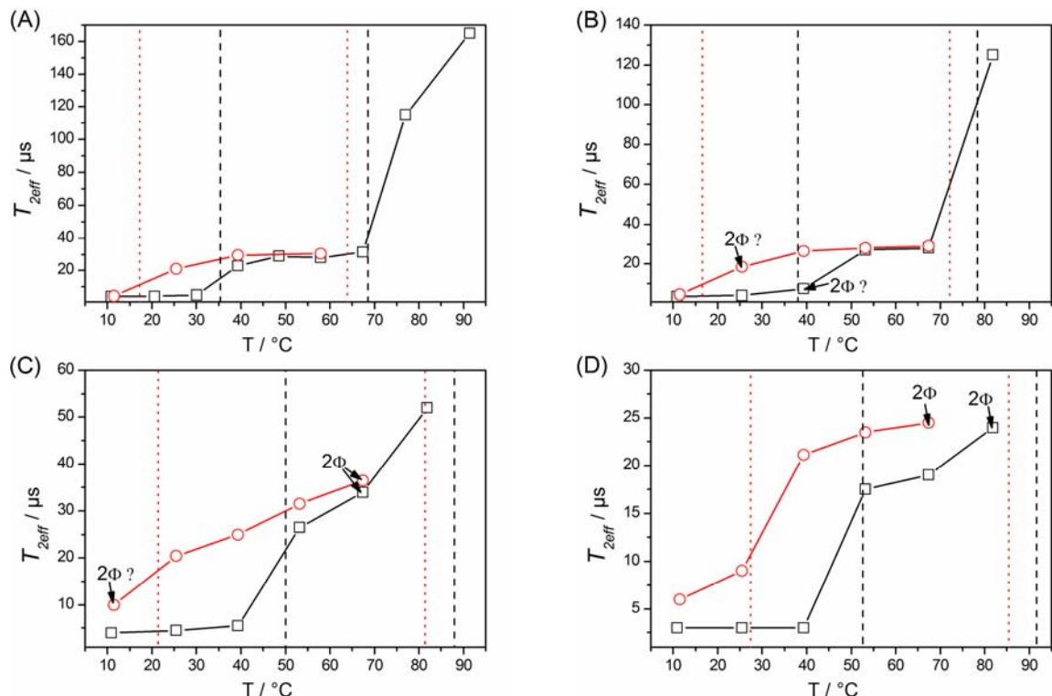
**Figure 6.** Variation of the decay constant  $T_2$  with temperature ((□) heating, (○) cooling) of ChC $m$  surfactants for  $m=12$  (A),  $m=14$  (B),  $m=16$  (C) and  $m=18$  (D). The black dashed vertical lines mark the transition temperatures on heating as detected by DSC, and the dotted red ones those on cooling (both for the first cycle).
