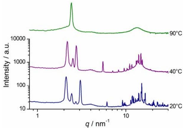
**Figure 7.** Small- and wide-angle X-ray scattering curves of neat ChC12 on raising temperature (freshly melted sample).
