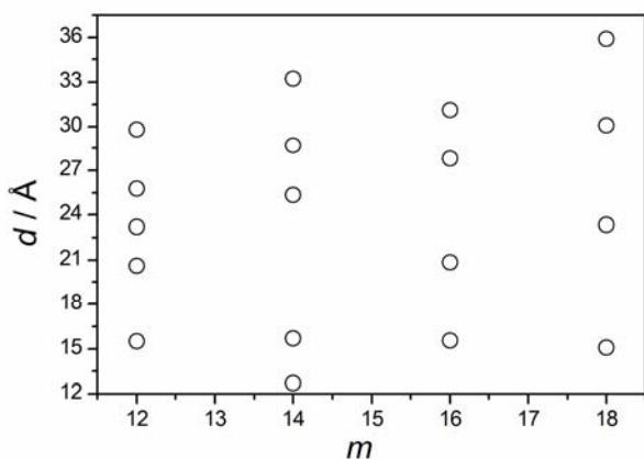
**Figure 11.** Comparison of the low-angle *d*-spacing values (up to  $q= 5 \text{ nm}^{-1}$ ) for different alkyl chain lengths ( $m= 12\text{-}18$ ) at low temperatures (20°C for  $m= 12$  and 18, 25°C for  $m= 16$ , and 30°C for  $m= 14$ ).
