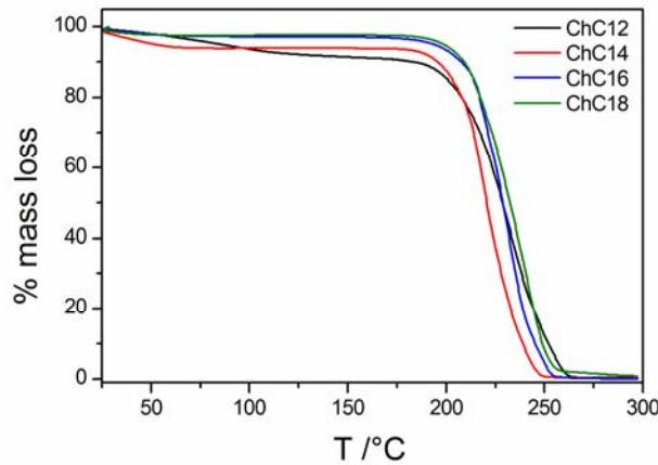
Figure 1. TGA curves of ChC<sub>m</sub> surfactants for  $m = 12-18$ .
