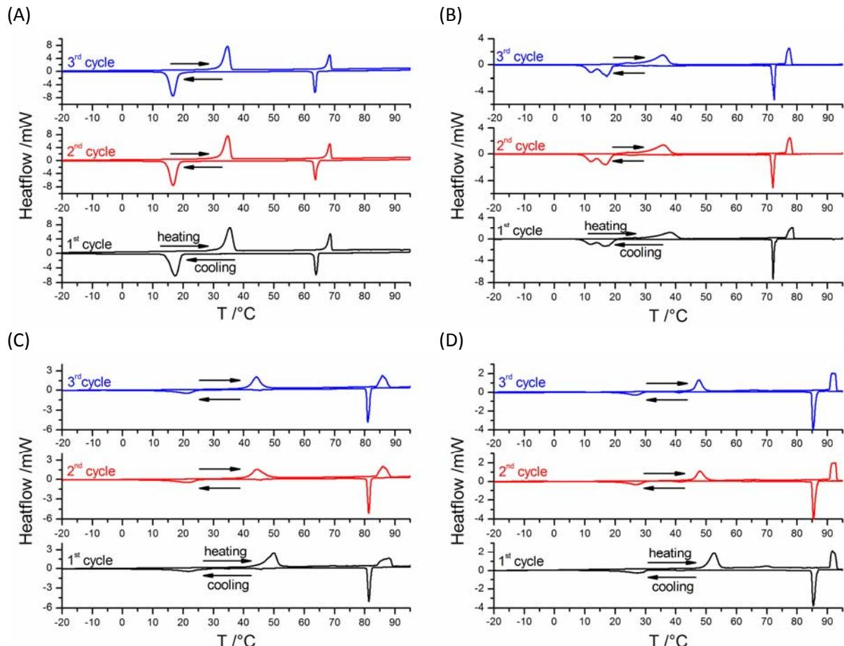
Figure 2. Three DSC cycles of ChC<sub>m</sub> surfactants between -20°C and 95°C:  $m = 12$  (A),  $m = 14$  (B),  $m = 16$  (C) and  $m = 18$  (D).
