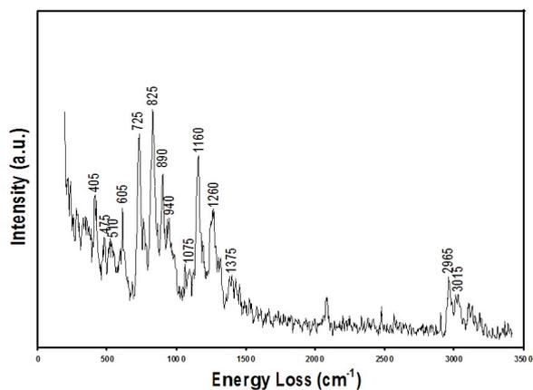
In-specular HREELS spectrum of sub-monolayer 2,2,2-trifluoroacetophenone on Pt(111) at 300 K.
