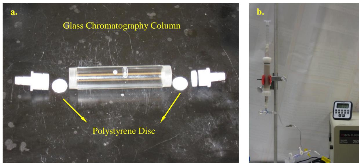
11 **Figure S1.** (a) Image of a 1.5 cm diameter, 6.8 cm long Omnifit glass chromatography column with 1.5
