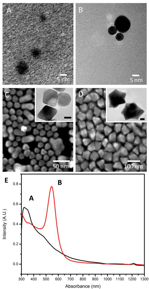
**Figure S2.** TEM images of Au seeds (A) freshly prepared and (B) after they are aged. SEM images, insets TEM images (scale bars 10 nm), of (C) Au cores prepared from freshly prepared Au seeds and (D) after the seeds were aged. In (E), the absorbance spectra for the freshly prepared and aged seeds, denoted A and B. The red-shift associated with the aged seeds is consistent with their larger size.
