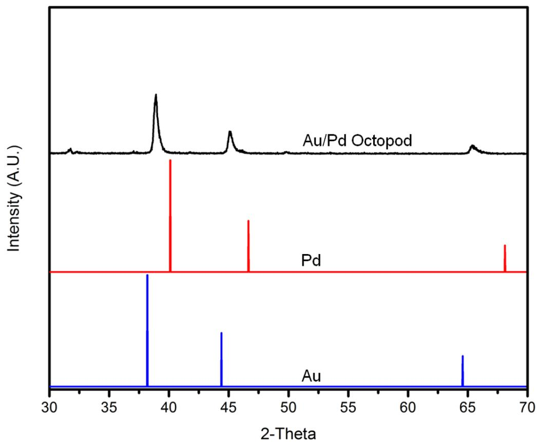
**Figure S3.** X-ray powder diffraction of Au/Pd octopods compared to Pd and Au standard cards. Peak positions are similar to those of Au as the Pd content is too low to give rise to distinct diffraction peaks. The shoulder peaks observed, however, can be attributed to Pd.
