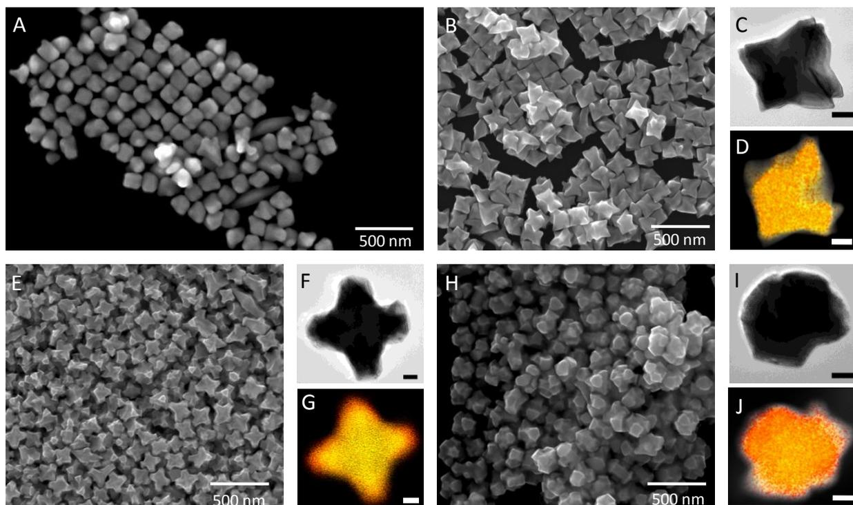
**Figure S4.** SEM (A, B, E, and H), TEM (C, F, and I) and STEM-EDX elemental mapping (D, G, and J) of Au/Pd nanoparticles, where yellow corresponds to Au and red corresponds to Pd. The Au:Pd mole ratio of precursors were: (A) 1-to-0, (B-D) 1-to-0.01, (E-G) 1-to-0.2, and (H-J) 1-to-0.5. Scale bars 25 nm (C, D, F, G, I, and J).
