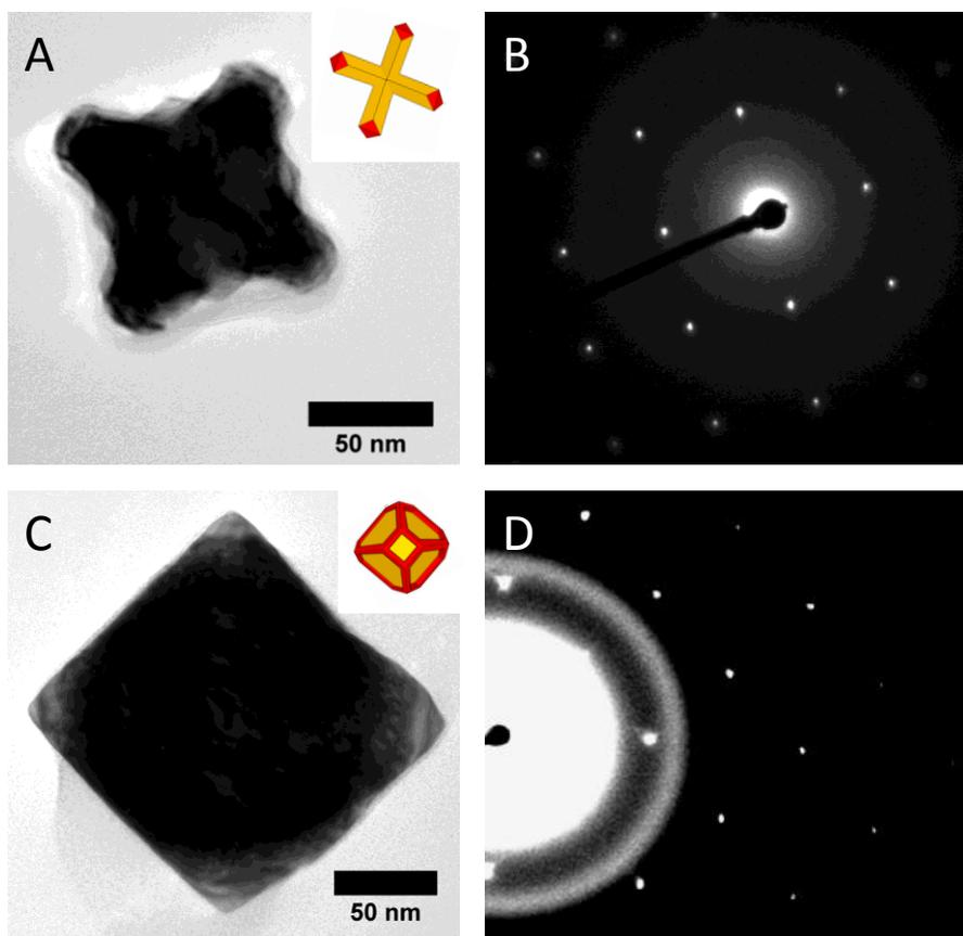
**Figure S1.** (A) TEM and (B) electron diffraction from an individual Au/Pd octopod oriented with four branches toward the substrate. (C) TEM and (D) electron diffraction from a concave Au@Pd cuboctahedron oriented with a (100)-terminating facet perpendicular to the electron beam.
