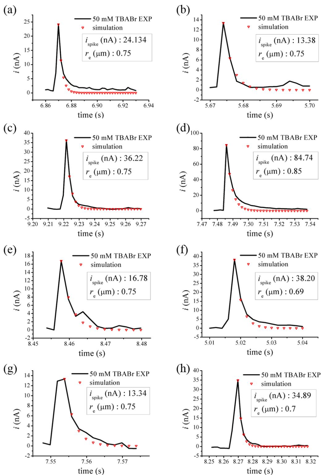
**Figure S20.** (a-h) The randomly chosen individual current spikes from a CA measured in a 0.5 M  $\text{H}_2\text{SO}_4$  aqueous solution containing 50 mM TBABr at a constantly applied potential of 1.2 V for 60 s. The purpose of fitting the bulk electrolysis model to the individual current spikes is to estimate the corresponding radius of an adsorbed hemispherical  $H\text{-TBABr}_3$  droplet.
