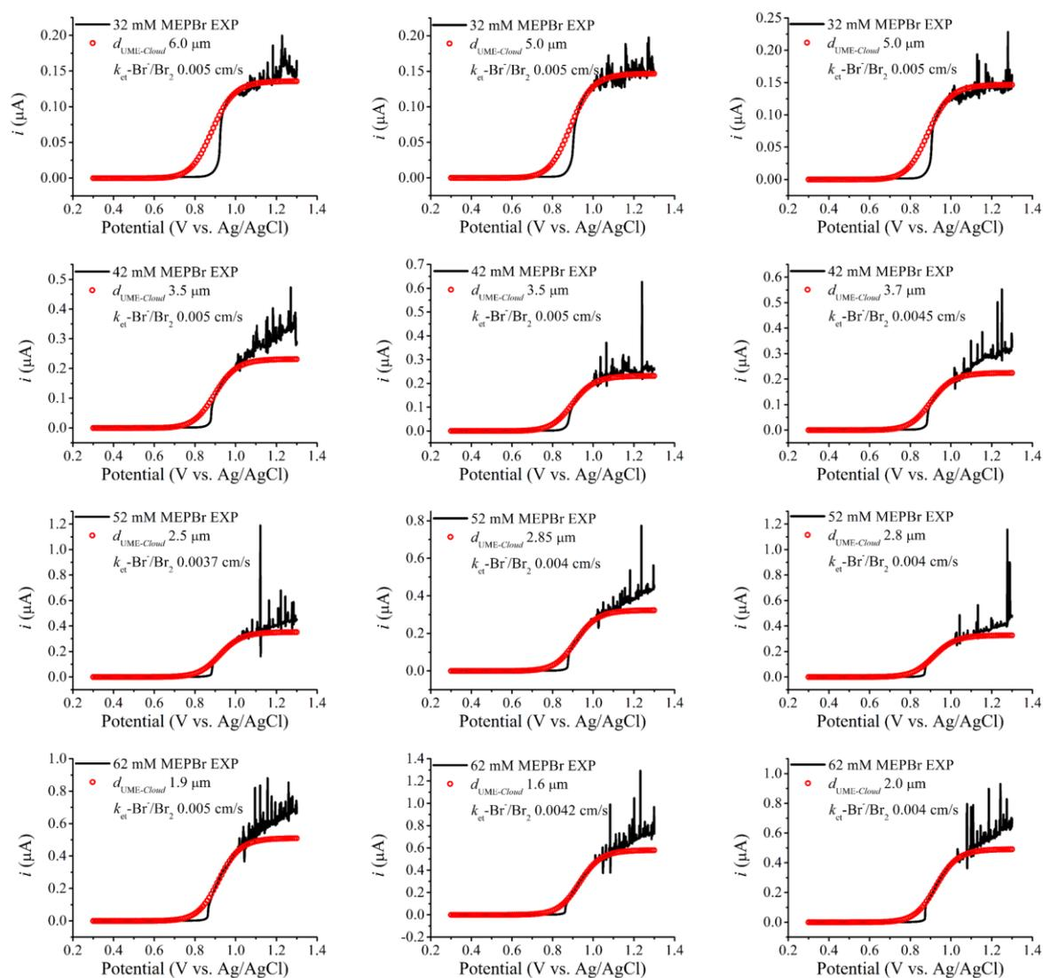
**Figure S6.** The linear sweep voltammograms (LSVs, black) measured in 0.5 M H<sub>2</sub>SO<sub>4</sub> aqueous solutions containing various concentrations of MEPBr (32, 42, 52, and 62 mM), and the corresponding simulation results (red) based on the *Cloud* model for the estimation of  $k_{\text{et}}\text{-Br}^-/\text{Br}_2$ .
