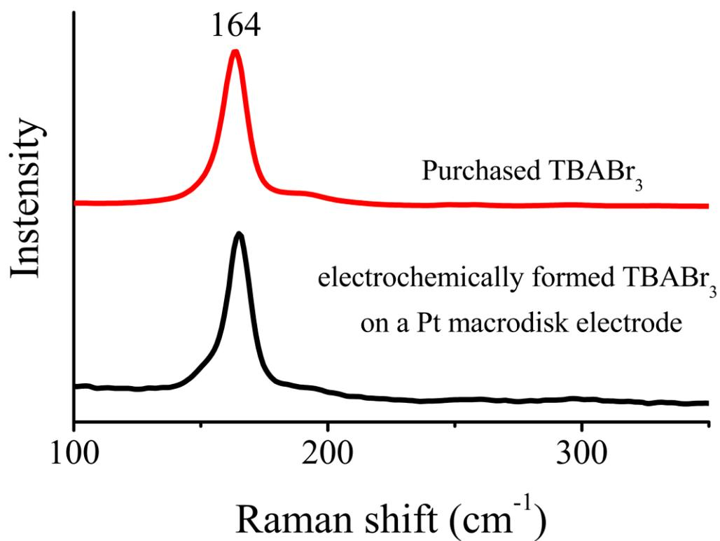
**Figure S2.** The Raman spectra measured from TBABr<sub>3</sub> formed electrochemically on a Pt macro disk electrode described in Figure S1 (black) and purchased from Sigma-Aldich (red).
