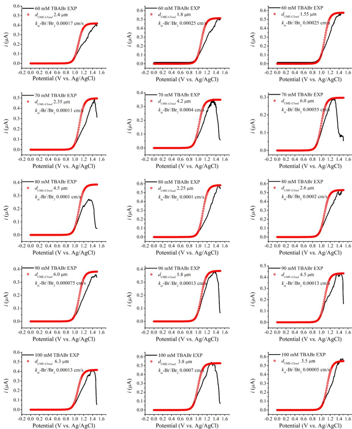
**Figure S14.** The LSVs (black) measured in 0.5 M H<sub>2</sub>SO<sub>4</sub> aqueous solutions containing various concentrations of TBABr (60, 70, 80, 90, and 100 mM), and the corresponding simulation results (red) based on the *Cloud* model for the estimation of  $k_{\text{et-Br}^-/\text{Br}_2}$ .
