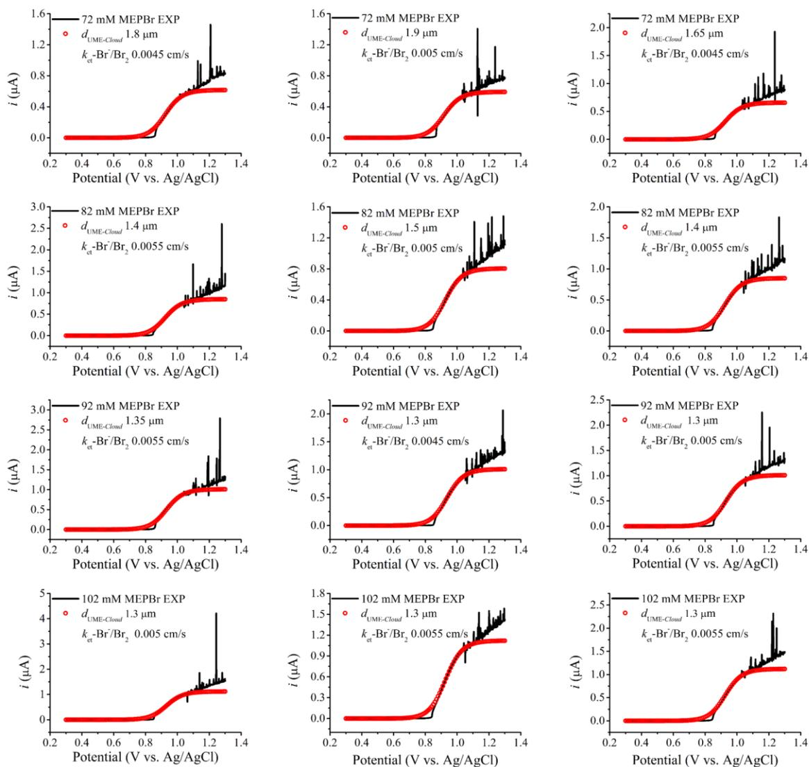
**Figure S7.** The LSVs (black) measured in 0.5 M H<sub>2</sub>SO<sub>4</sub> aqueous solutions containing various concentrations of MEPBr (72, 82, 92, and 102 mM), and the corresponding simulation results (red) based on the *Cloud* model for the estimation of  $k_{et-Br^-/Br_2}$ .
