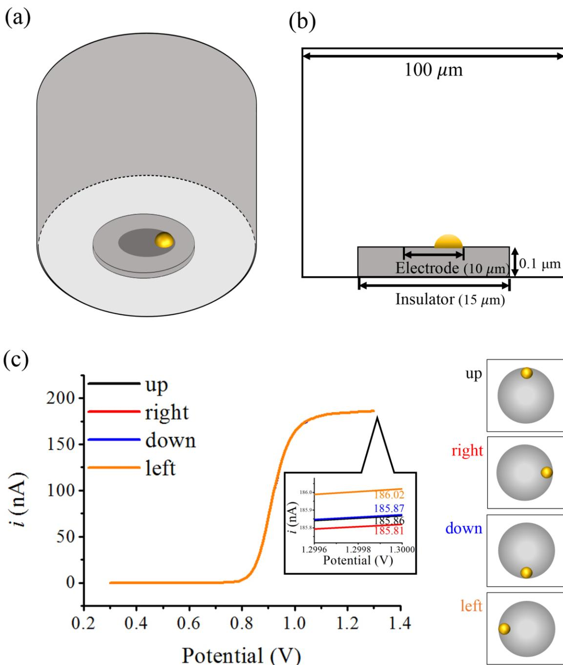
**Figure S19.** (a) Three dimensional, (b) the corresponding cross-sectional domain of the simulation, and (c) simulated, normalized steady-state voltammograms under the different conditions. IP adsorbed on different UME edge sites.
