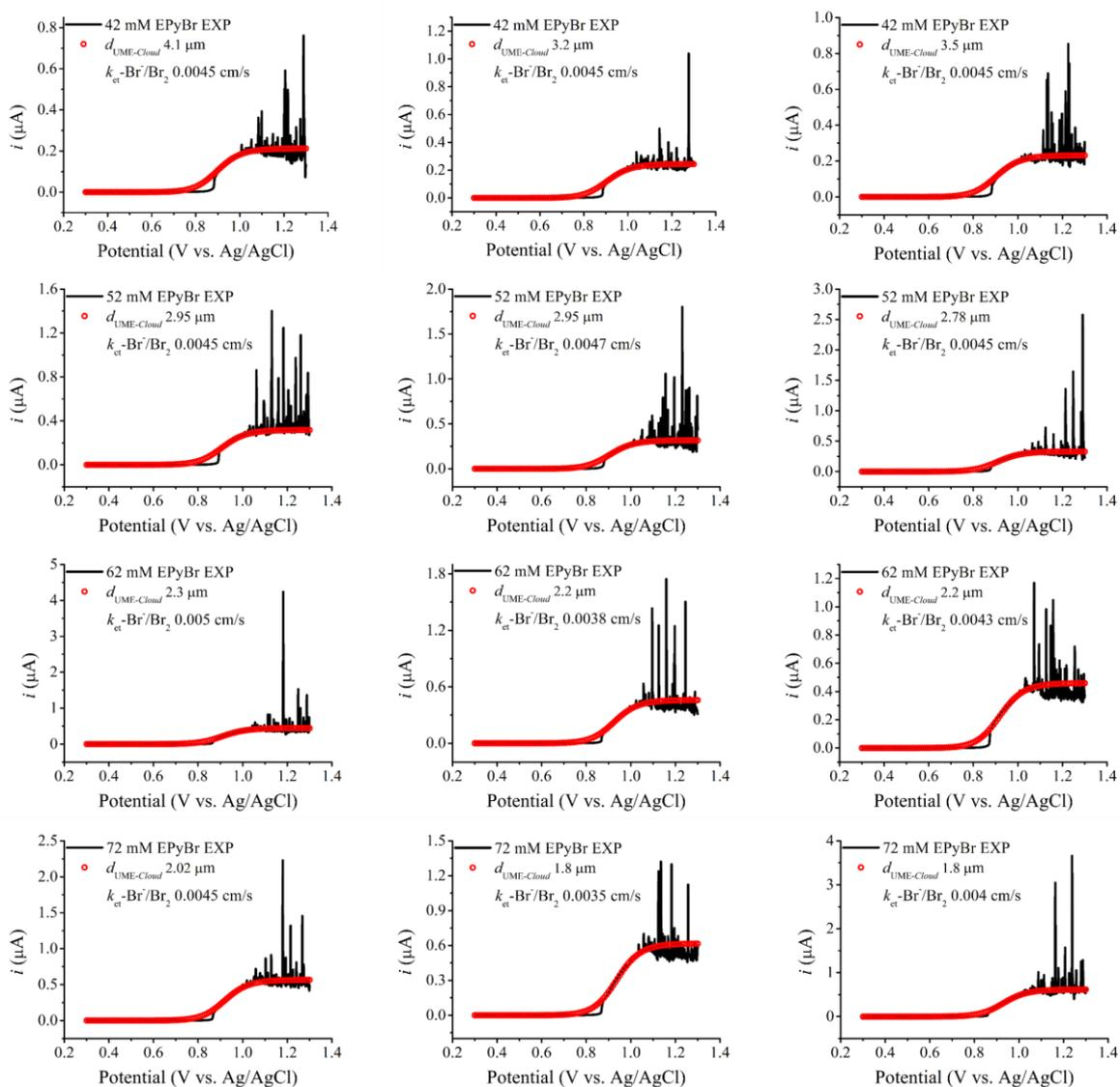
**Figure S9.** The LSVs (black) measured in 0.5 M  $\text{H}_2\text{SO}_4$  aqueous solutions containing various concentrations of EPyBr (42, 52, 62, and 72 mM), and the corresponding simulation results (red) based on the *Cloud* model for the estimation of  $k_{\text{et-Br}^-/\text{Br}_2}$ .
