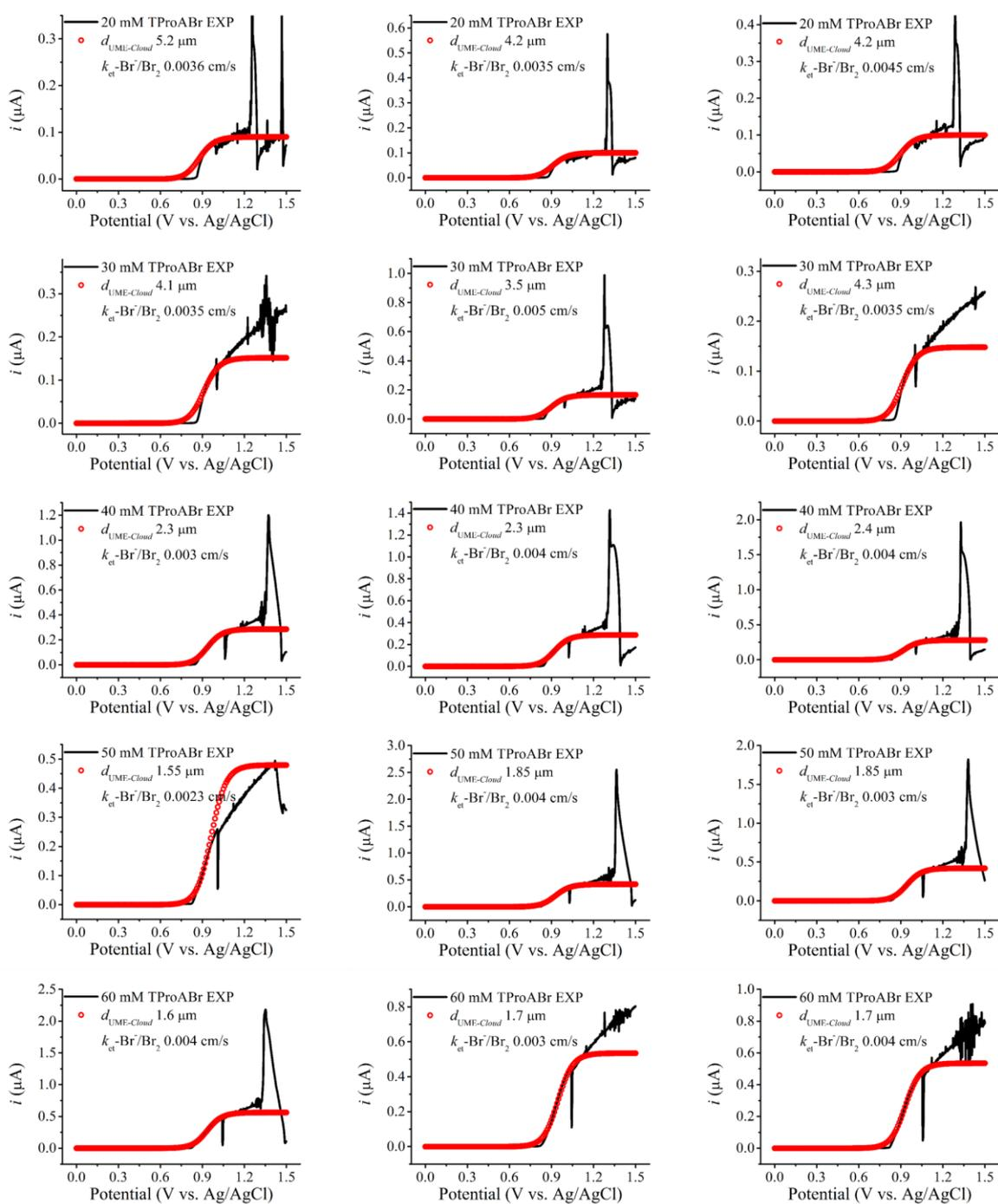
**Figure S11.** The LSVs (black) measured in 0.5 M  $\text{H}_2\text{SO}_4$  aqueous solutions containing various concentrations of TProABr (20, 30, 40, 50, and 60 mM), and the corresponding simulation results (red) based on the *Cloud* model for the estimation of  $k_{\text{et}}\text{-Br}^-/\text{Br}_2$ .
