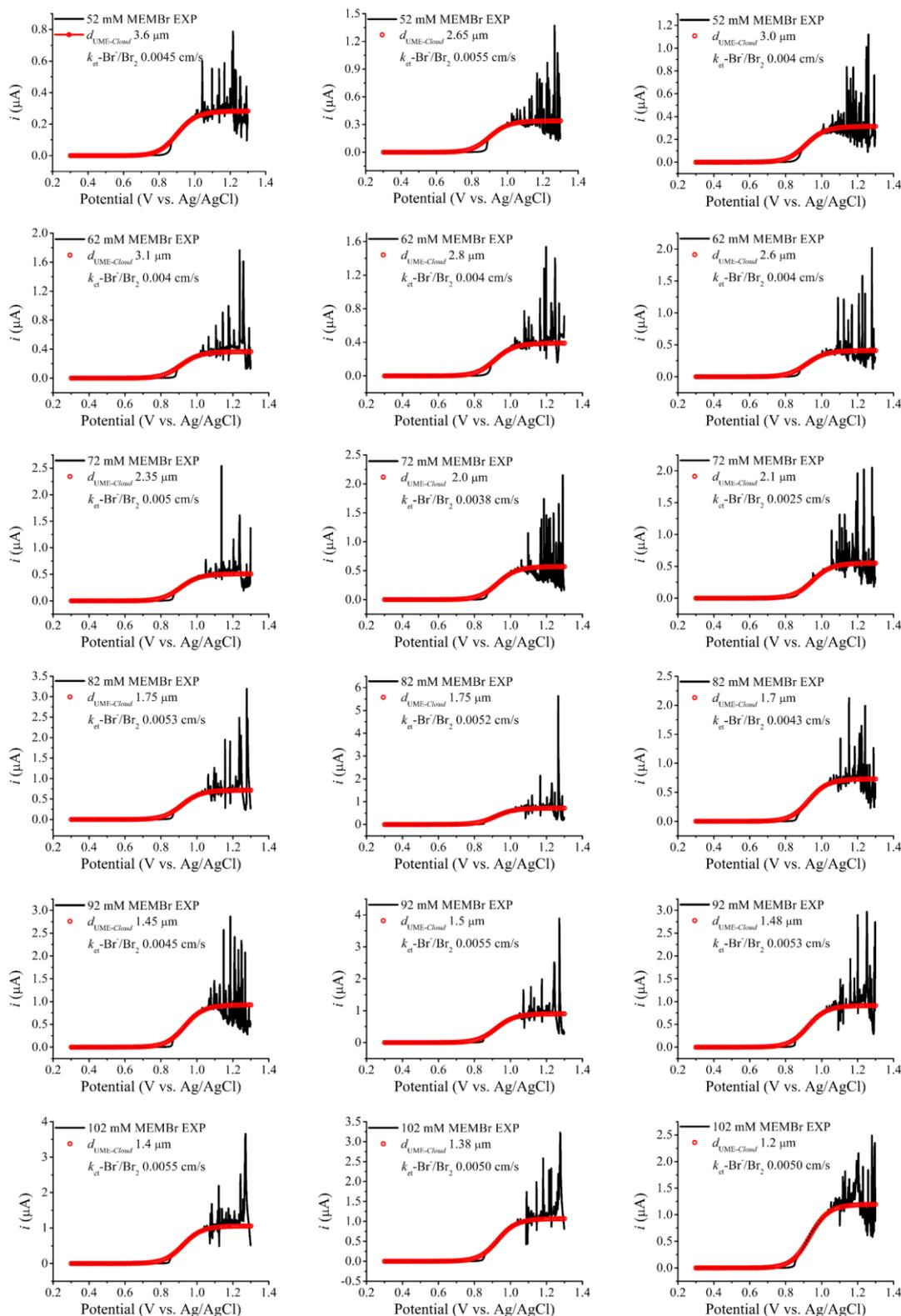
**Figure S8.** The LSVs (black) measured in 0.5 M H<sub>2</sub>SO<sub>4</sub> aqueous solutions containing various concentrations of MEMBr (52, 62, 72, 82, 92, and 102 mM), and the corresponding simulation results (red) based on the *Cloud* model for the estimation of  $k_{\text{et-Br}^-/\text{Br}_2}$ .
