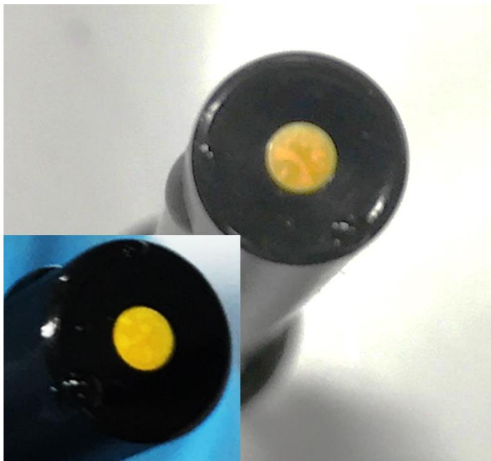
**Figure S1.** The photograph of precipitated TBABr<sub>3</sub> on a Pt macro disk electrode with a radius of 1 mm after a potential of 1.5 V was applied for 1000 s in a 0.5 M H<sub>2</sub>SO<sub>4</sub> aqueous solution with  $C_{\text{TBABr}} = 50$  mM.
