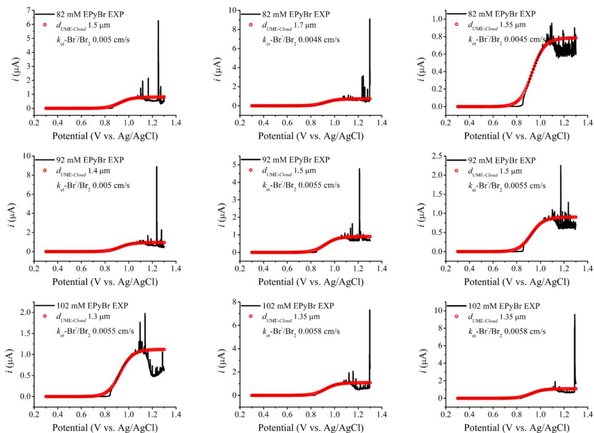
**Figure S10.** The LSVs (black) measured in 0.5 M  $\text{H}_2\text{SO}_4$  aqueous solutions containing various concentrations of EPyBr (82, 92, and 102 mM), and the corresponding simulation results (red) based on the *Cloud* model for the estimation of  $k_{\text{et-Br}^-/\text{Br}_2}$ .
