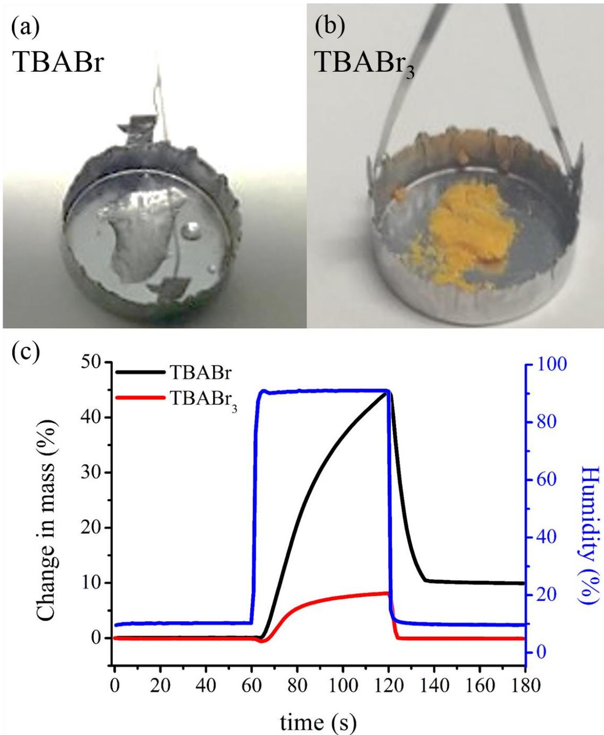
**Figure S17.** The photographs of (a) TBABr and (b) TBABr<sub>3</sub> after the dynamic vapor sorption (DVS) analysis, which is depicted in (c); the graph describes change in mass (%) of TBABr (black) and TBABr<sub>3</sub> (red) powder as humidity changes (blue line) from 0 to 90 %.
