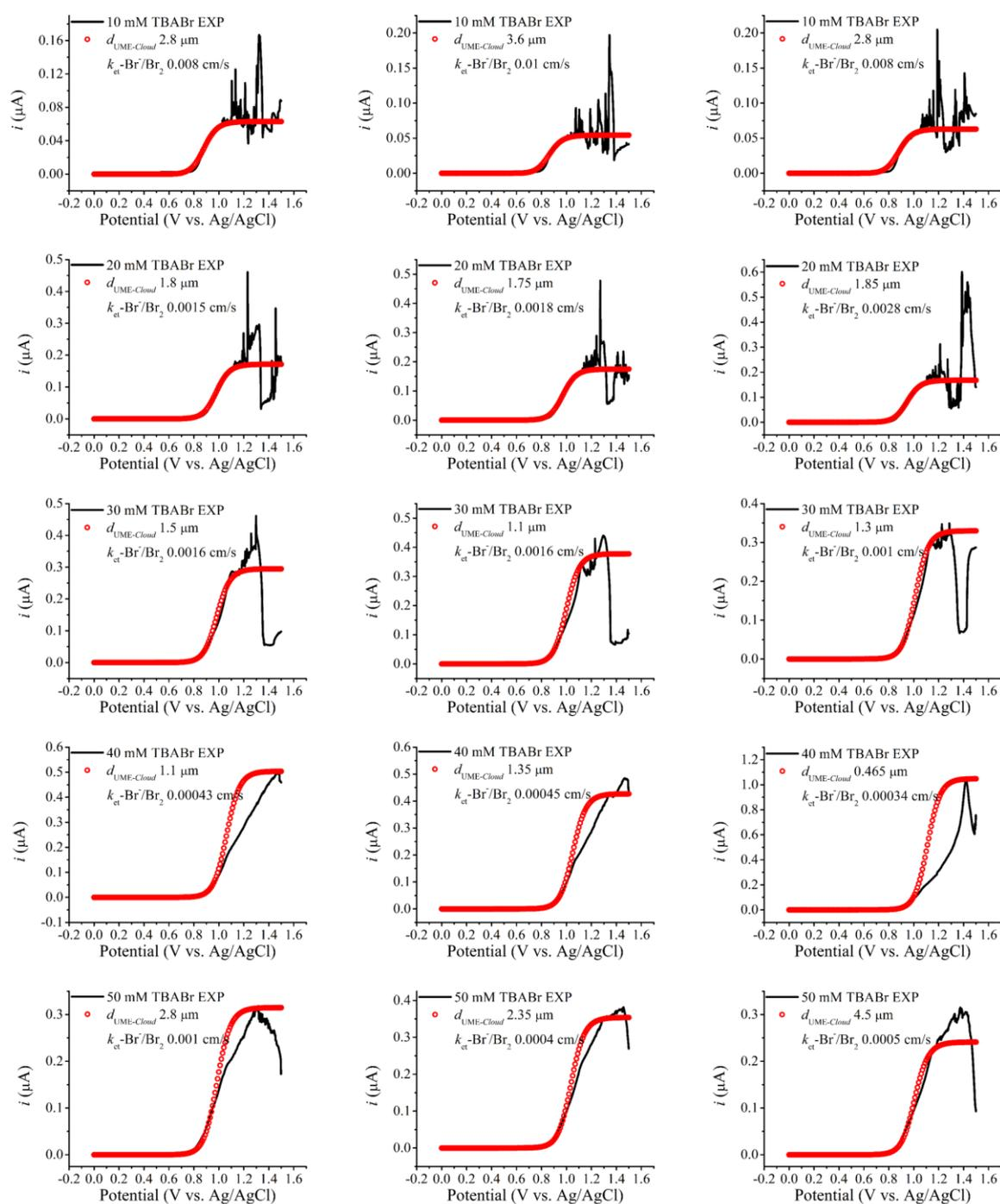
**Figure S13.** The LSVs (black) measured in 0.5 M H<sub>2</sub>SO<sub>4</sub> aqueous solutions containing various concentrations of TBABr (10, 20, 30, 40, and 50 mM), and the corresponding simulation results (red) based on the *Cloud* model for the estimation of  $k_{\text{et-Br}^-/\text{Br}_2}$ .
