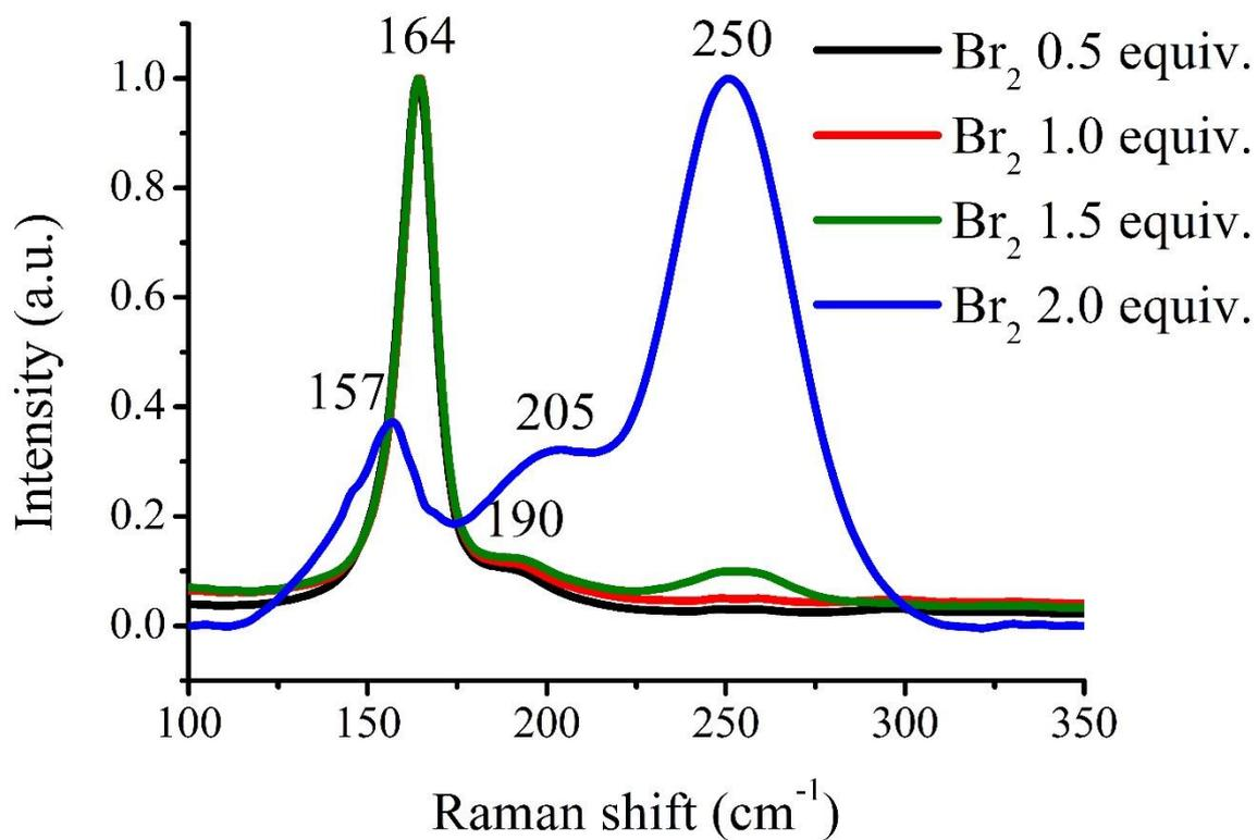
**Figure S4.** The Raman spectra obtained from  $\text{TBr}_{2n+1}$ , which were chemically synthesized by adding  $\text{Br}_2$  to  $\text{TBr}$  aqueous solutions to have different ratios of  $C_{\text{Br}_2(aq)}$  to  $C_{\text{Br}^-(aq)}$ .
