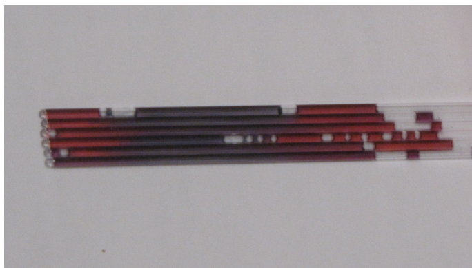
Figure S7. Photo of LED capillary tubes containing sec -phenethyl alcohol, \text{H}_2\text{O}_2 and AuNP following 20 minutes of irradiation. Note deep violet color in the areas exposed to LED light.
