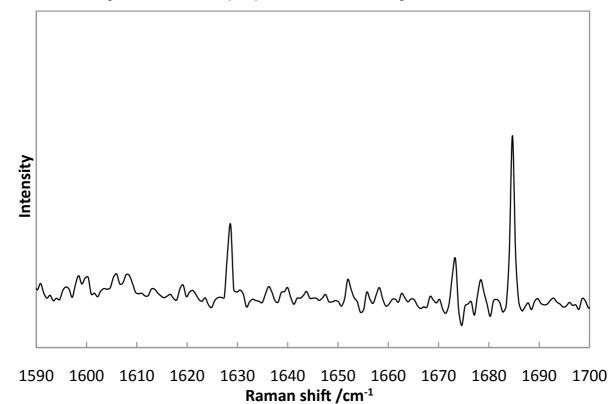
The secondary structure of the  $(LE)_8$ -PEG<sub>70</sub> peptide monolayer was measured by SERS spectroscopy. The monolayer was formed on a gold-nanoparticle- coated glass substrate. The excitation wavelength was 532.1 nm. The peaks at 1628 and 1685 cm<sup>-1</sup> were assigned to amide I of the antiparallel  $\beta$ -sheet and the  $\beta$ -plated sheet, respectively.
