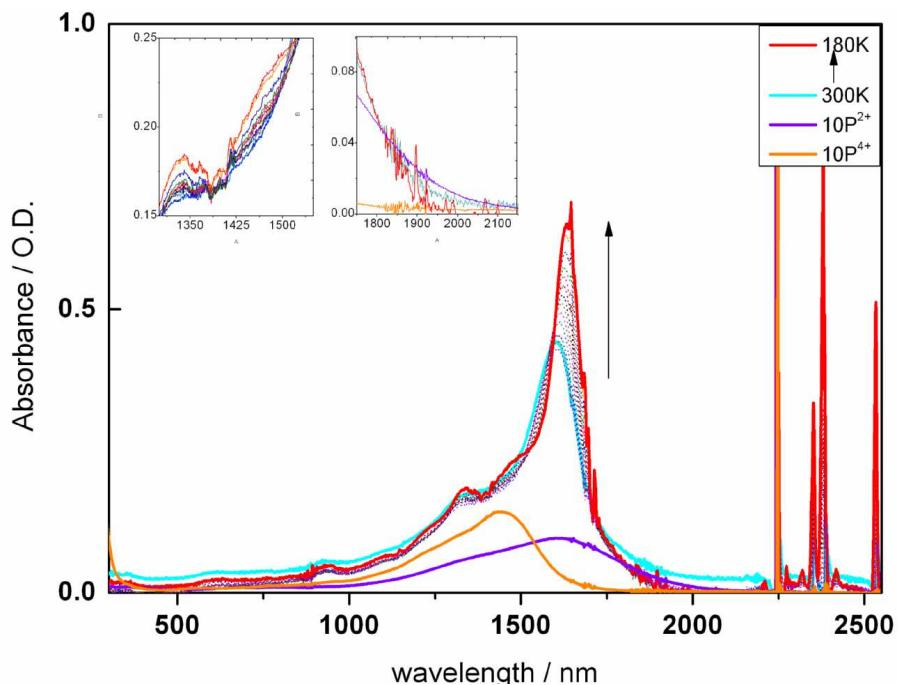
**Figure S5.** Change in absorption spectra upon cooling of  $\text{CH}_2\text{Cl}_2$  solutions of (a)  $\text{10P}_{\text{Hex}}^{3+}$  generated by the reaction of  $\text{10P}_{\text{Hex}}$  with 4.5 equivalents of  $\text{SbCl}_5$ .
