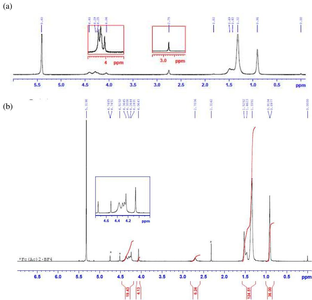
**Figure S7.**  $^1\text{H}$  NMR spectra of (a)  $\mathbf{6P}_{\text{Hex}}^{2+}$  at 210 K and (d)  $\mathbf{6P}_{\text{Hex}}^{2+}$  at room temperature in the presence of  $\text{Fe}(\text{C}_5\text{H}_4\text{Ac})_2 \cdot \text{AgBF}_4$  in  $\text{CD}_2\text{Cl}_2$ .
