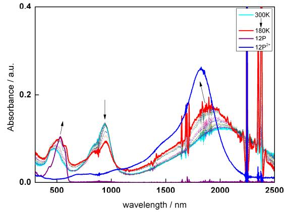
**Figure S4.** Change in absorption spectra upon cooling of  $\text{CH}_2\text{Cl}_2$  solutions of (a)  $\text{4P}_{\text{Hex}}^+$  ( $33.2 \mu\text{M}$ ), (b)  $\text{10P}_{\text{Hex}}^+$  ( $16.9 \mu\text{M}$ ), and (c)  $\text{12P}_{\text{Hex}}^+$  ( $16.5 \mu\text{M}$ ) generated by the reaction of the corresponding neutral species with 1.5 equivalents of  $\text{SbCl}_5$ .
