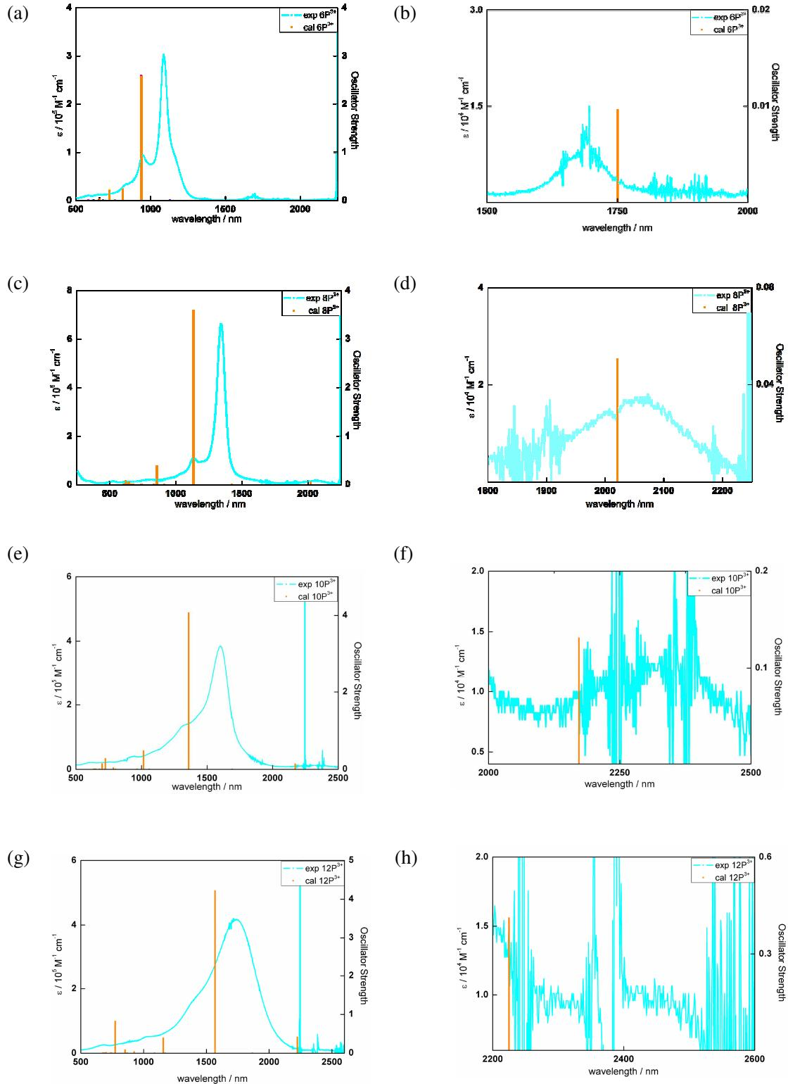
**Figure S2.** Observed UV-vis-NIR spectra of  $n\text{P}_{\text{Hex}}^{3+}$  and calculated excitation energy of  $n\text{P}_\text{H}^{3+}$  at the TD-B3LYP/6-31G(d) level ((a) (b)  $n = 6$ , (c) (d)  $n = 8$ , (e) (f)  $n = 10$ , and (g) (h)  $n = 12$ ). The heights of the calculated spectra reflect the calculated oscillator strengths.
