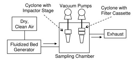
Figure S2. Experimental setup for the loading tests to evaluate the impactor's performance.
