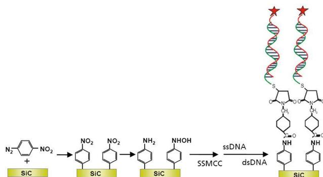
**Scheme 1.** Schematic plot of bio-functionalization of SiC with DNA. The term of SSMCC stands for the cross-linker of sulphosuccinimidyl-4-(N-maleimidomethyl) cyclohexane-1-carboxylate.
