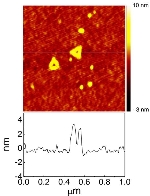
**Figure S3.** High magnification AFM image and cross section of triangular ridges produced upon exposure of DNA origami triangles on SiO<sub>2</sub> surface to HF vapor under low moisture condition.
