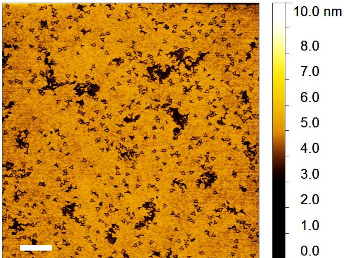
**Figure S1.** AFM image of triangular trenches produced upon exposure of DNA origami triangles on SiO<sub>2</sub> surface to HF vapor under high moisture condition. Scale bar 500 nm.
