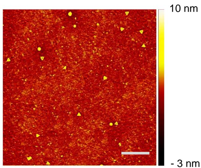
**Figure S2.** AFM image of triangular ridges produced upon exposure of DNA origami triangles on  $\text{SiO}_2$  surface to HF vapor under low moisture condition. Scale bar 1  $\mu\text{m}$ .
