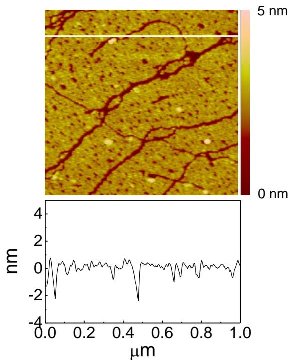
**Figure S4.** High magnification AFM image and cross section of trenches produced upon exposure of  $\lambda$ -DNA aligned on  $\text{SiO}_2$  surface to HF vapor under high moisture conditions.
