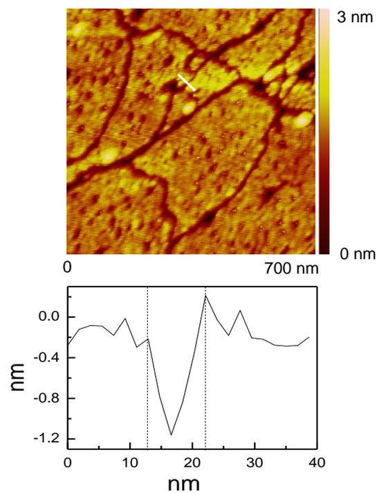
**Figure S5.** High magnification AFM image and the cross section of a trench showing width of  $\sim 5$  nm (FWHM). The white line in the figure indicates location of the cross section.
