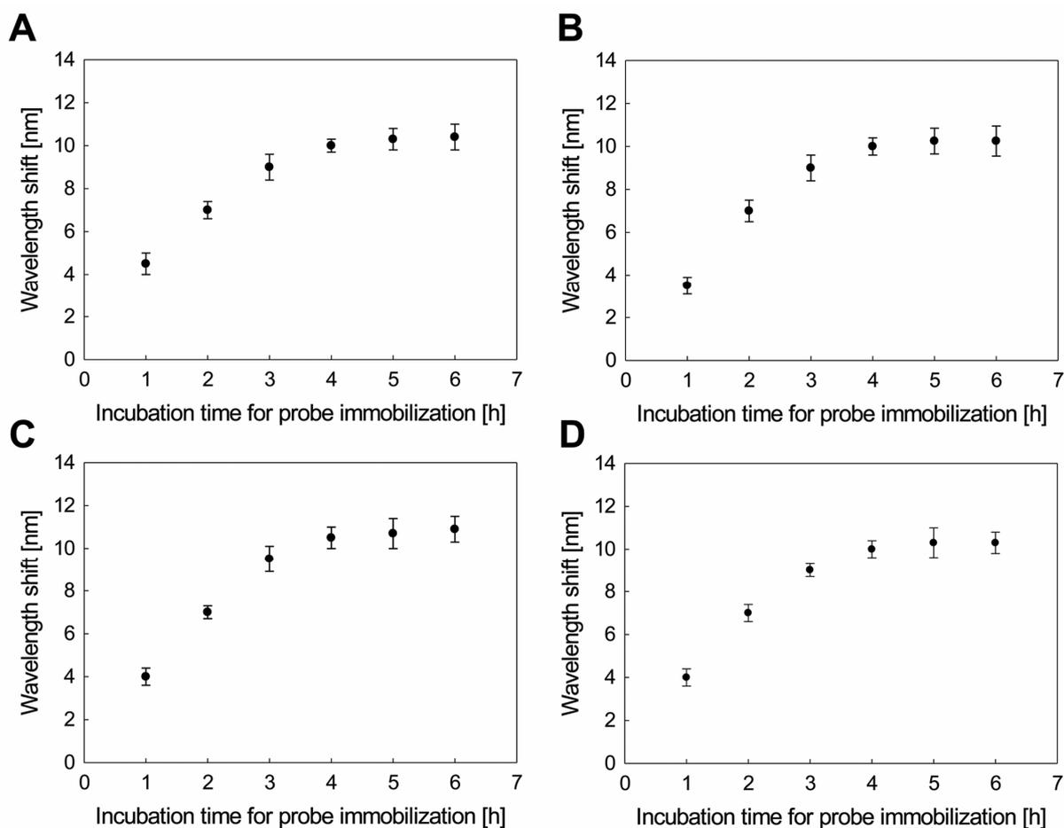
**Figure S6.** Effect of the incubation time for the immobilization of probe DNAs on the LSPR wavelength shift. The 10  $\mu$ M probe DNAs were treated on the MC-NPA chip for the different incubation time (1, 2, 3, 4, 5 and 6 h, respectively), and then hybridized with target DNAs, (A) Efm003-20, (B) Sau001-20, (C) Smal03-20 and (D) Vvul02-20, respectively. The data were obtained from three measurements and the error bars represent standard deviation.
