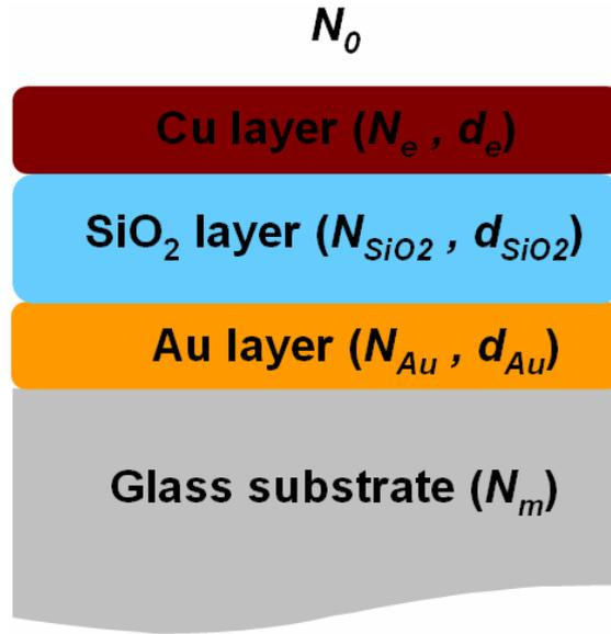
**Figure S3.** Schematic diagram illustrating the multilayer model for the description of simulation data from Cu-layer/SiO<sub>2</sub>-layer/Au-layer/glass substrate composite structures. Here,  $N$  is a refractive index (RI) and  $d$  is a thickness of each layer. The RI of a porous Cu film is calculated by using Maxwell-Garnett effective medium theory. Reflection and extinction spectra can be also calculated by using the characteristic matrix of each layer.
