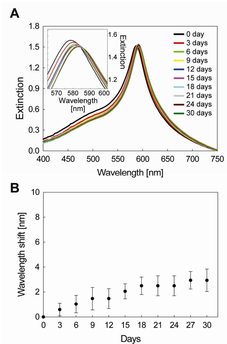
**Figure S4.** Stability test of MC-NPA chips under ambient condition. MC-NPA chip was incubated at RT with 30% humidity for 30 days and the LSPR spectrum were measured once every three days. (A) Spectrum profiles of MC-NPA chip is shown in the left illustrations and are magnified (inset). (B) Plot of wavelength shift versus incubation day.
