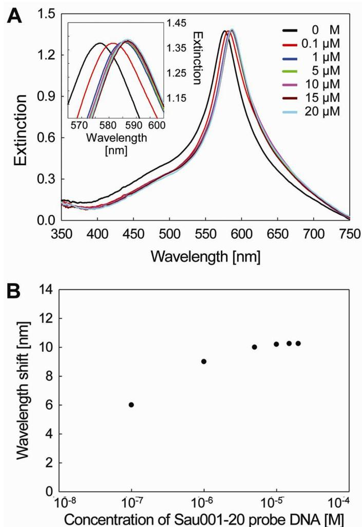
**Figure S5.** Effect for the concentration of probe DNAs on the LSPR wavelength shift. The spots of MC-NPA chip were assembled with the different concentration of probe DNAs (20, 15, 10, 5, 1 and 0.1  $\mu$ M, respectively) and then hybridized with target DNAs. (A) LSPR Spectrum profiles of chips and the magnified spectrum profiles (inset). (B) Plot of LSPR wavelength shift versus the concentration of probe DNA.
