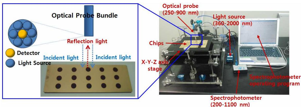
**Figure S2.** Experimental setup and the optical measurement system for the LSPR-based MC-NPA chip. The optical measurement system for the evaluation of the optical properties on the MC-NPA chip was based on a spectroscopy system.
