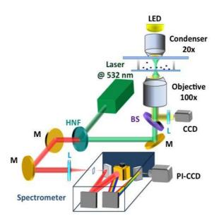
Figure 1: Schematic of the experimental set-up used for SERS analysis. Abbreviations: M, mirror; L, lens; HNF, holographic notch filter; BS, beam splitter; CCD, Charge Coupled Device.
