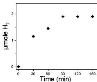
**Figure S3.** Time course for H<sub>2</sub> production from a 80 nM *S. leopoliensis* PSI-cobaloxime solution.
