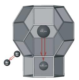
Presence of  $Ru^{3+}$  on SI was found to affect the position of SIII cations. Under oxidising conditions  $Ru^{3+}$  was found in the centre of D6R with SIII (occupied by  $Na^+$ ) moved far into the sc. Reduction of  $Ru^{3+}$  caused its migration into sod. In this case SIII was found significantly closer to the framework.
