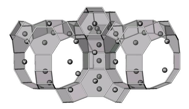
SI: centre of double 6-ring (D6R). Occupied by  $Ru^{3+}$  during NOx adsorption under oxidising conditions
