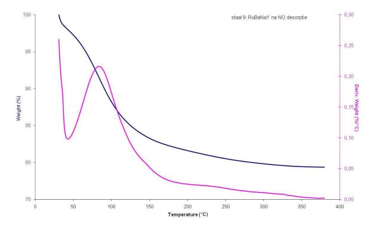
The weight loss above 150°C corresponded to 31 water molecules in very good agreement with the 32 water molecules determined by Rietveld refinement. The earlier onset of dehydration during TG was caused by the dry environment while  $NO_x$  adsorption/desorption always occurred in presence of water.
