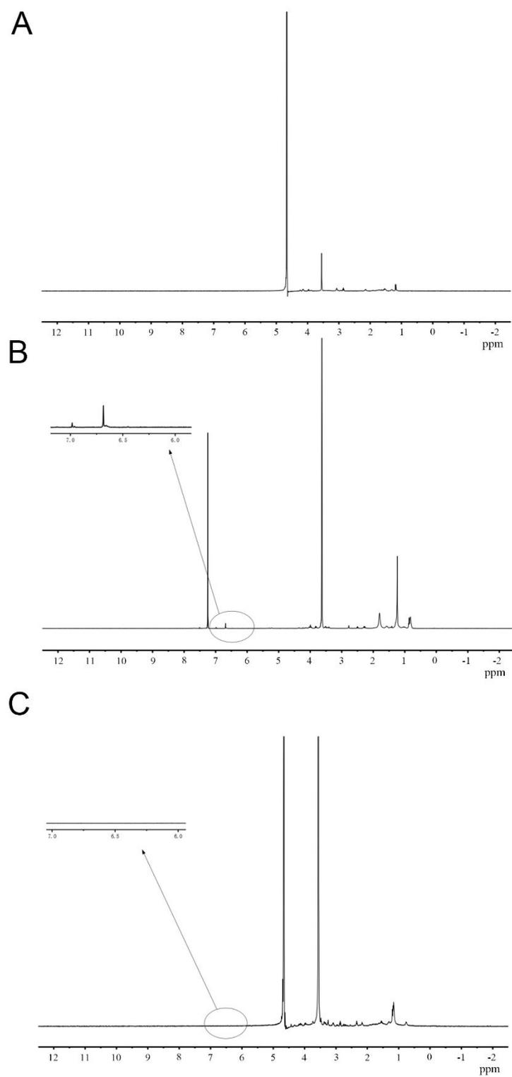
**Figure S1** <sup>1</sup>H-NMR spectrum of (A) CREKA (B) Mal-PEG<sub>2000</sub>-DSPE and (C) CREKA-PEG<sub>2000</sub>-DSPE
