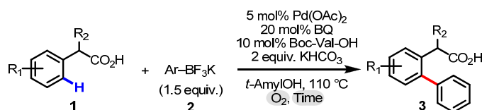
Scheme S2: General procedure for C–H/organoboron cross-coupling under aerobic conditions.
