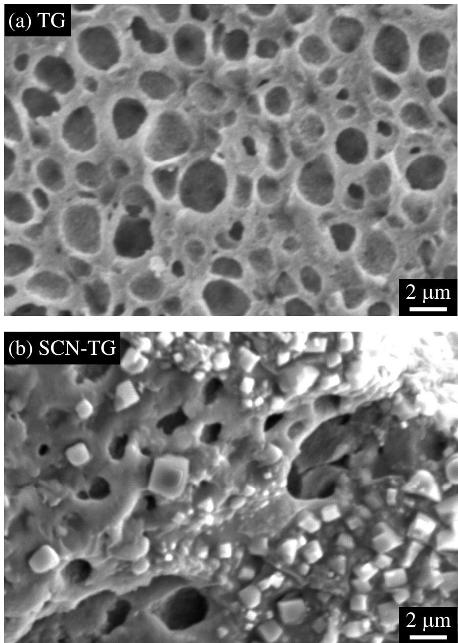
**Figure S1.** SEM images of the tannin gel surfaces before and after  $\text{SCN}^-$  loading: (a) tannin gel (TG); (b)  $\text{SCN}^-$ -retaining tannin gel (SCN-TG).
