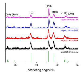
XRD spectra for powder samples of  $Cu_{2-x}S$  nanodisks that possess different aspect-ratios. As aspect ratioincreases, the relative intensity of the diffraction peak corresponding to the (110) plane increases.
