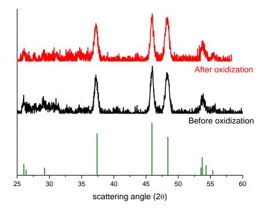
XRD spectra for powder samples of the nanodisks before and after thermal oxidation. After oxidation, a small decrease is observed in the relative intensity of the peak corresponding to the (110) crystal plane.
