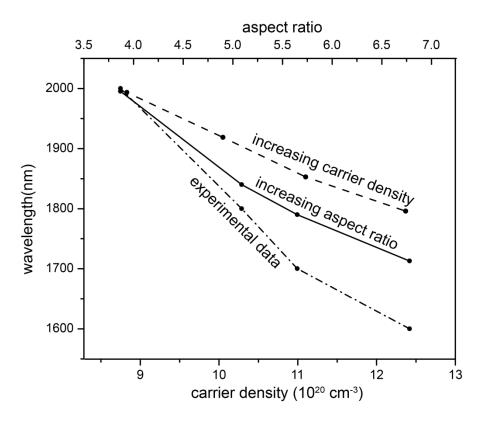
The calculated change in LSPR wavelength for the out-of-plane mode for nanodisks with independently increasing aspect ratios (solid) and carrier densities (dashed), compared to the experimental data (dotdash) obtained from the spectra in Figure 2a.
