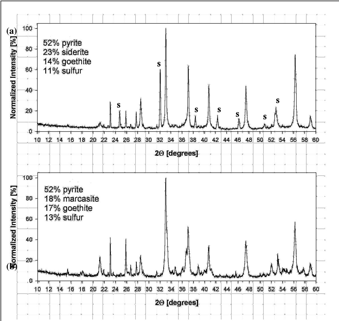
44 **Figure S3.** XRD patterns associated with the product formed via the reaction of (a) lepidocrocite
