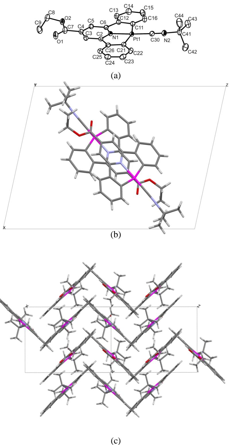
Figure S3. a) ORTEP view of **5**. Ellipsoids are drawn at 50% probability level. Hydrogen atoms and solvent molecules have been omitted for clarity; b) View along *b* axis of the head to tail molecular pairs. These molecular pairs show  $\pi\cdots\pi$  contacts (3.38–3.63 Å) between the aromatic rings of the CNC ligand. c) Crystal-packing showing molecular piles in a zig-zag network.
