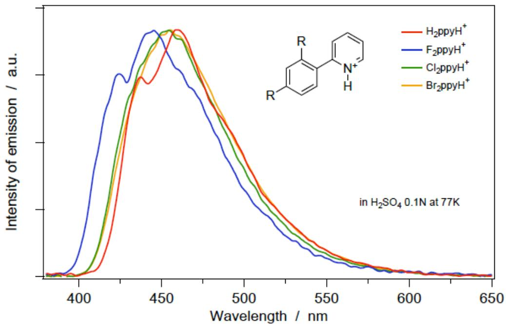
**Figure S6.** Normalized phosphorescence spectra of the protonated forms of the 2-(2,4-di-X-phenyl)pyridines ( $X = \text{H}, \text{F}, \text{Cl}, \text{Br}$ ) in 0.1 N  $\text{H}_2\text{SO}_4$  at 77 K ( $\lambda_{\text{exc}} = 285$  nm, 10  $\mu\text{s}$  delay).
