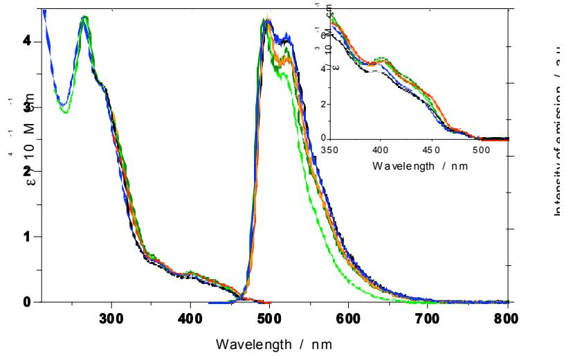
**Figure S2.** Absorption (left) and emission (right) spectra of **ClIrPic** at 298 K in different solvents: dimethyl sulfoxide (black), acetonitrile (blue), chloroform (olive), dichloromethane (green), 1,2-dichlorobenzene (orange) and toluene (red). The absorption spectral window between 350 and 525 nm is magnified in the inset for the sake of clarity. Emission spectra ( $\lambda_{exc} = 407$  nm) are corrected for the detector response.
