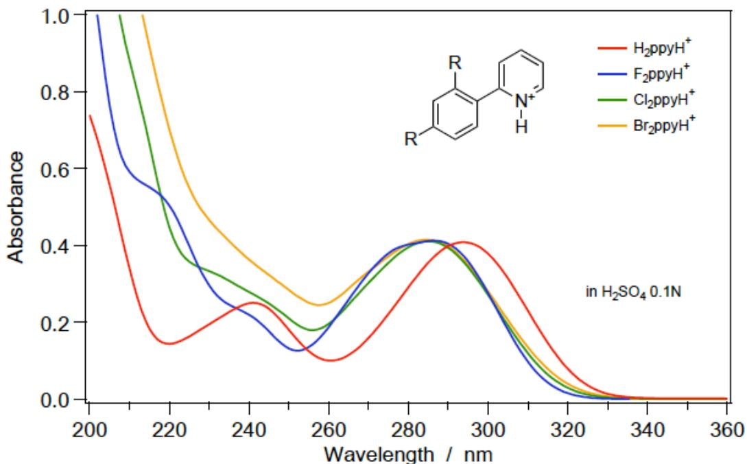
**Figure S4.** Normalized absorption spectra of the protonated forms of the 2-(2,4-di-X-phenyl)pyridines ( $X = \text{H}, \text{F}, \text{Cl}, \text{Br}$ ) in 0.1 N  $\text{H}_2\text{SO}_4$  at room temperature.
