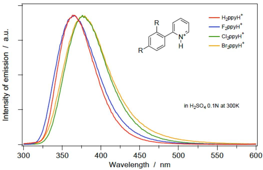
**Figure S5.** Normalized fluorescence spectra of the protonated forms of the 2-(2,4-di-X-phenyl)pyridines ( $X = \text{H}, \text{F}, \text{Cl}, \text{Br}$ ) in 0.1 N  $\text{H}_2\text{SO}_4$  at room-temperature ( $\lambda_{\text{exc}} = 285$  nm).
