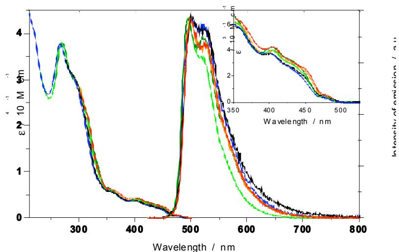
**Figure S3.** Absorption (left) and emission (right) spectra of **BrIrPic** at 298 K in different solvents: dimethyl sulfoxide (black), acetonitrile (blue), chloroform (olive), dichloromethane (green), 1,2-dichlorobenzene (orange) and toluene (red). The absorption spectral window between 350 and 525 nm is magnified in the inset for the sake of clarity. Emission spectra ( $\lambda_{\text{exc}} = 407 \text{ nm}$ ) are corrected for the detector response.
