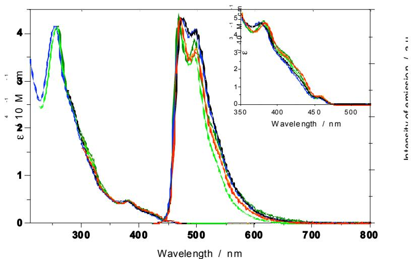
**Figure S1.** Absorption (left) and emission (right) spectra of **FIrPic** at 298 K in different solvents: dimethyl sulfoxide (black), acetonitrile (blue), chloroform (olive), dichloromethane (green), 1,2-dichlorobenzene (orange) and toluene (red). The absorption spectral window between 350 and 525 nm is magnified in the inset for the sake of clarity. Emission spectra ( $\lambda_{exc} = 407$  nm) are corrected for the detector response.
