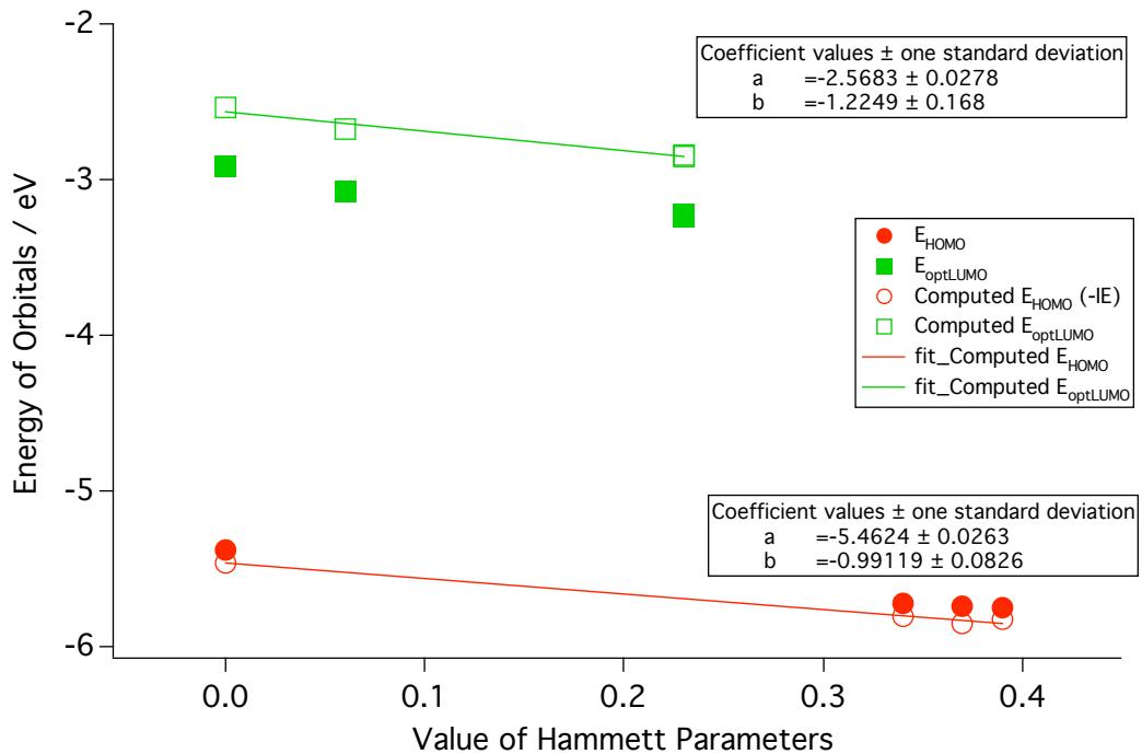
**Figure S7.** Correlation between the orbital energy levels (experimental and computed) and Hammett parameters.  $E_{optLUMO}$  is correlated with the values  $\sigma_p$  and  $E_{HOMO}$  (-IE) with the values  $\sigma_m$ . Fits are of the form  $y=a+bx$ .
