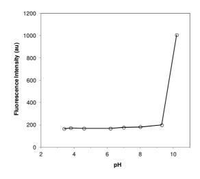
**Fig. S3** Fluorescence intensity ( $\lambda_{ex}/\lambda_{em} = 570/594$  nm, slit widths 2.5 nm) of probe **1** (1.0  $\mu$ M in pure water) vs pH variation at room temperature.
