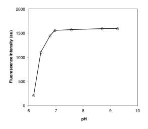
**Fig. S6** The variation of fluorescence intensity ( $\lambda_{ex}/\lambda_{em} = 570/594$  nm, slit widths 2.5 nm) of probe 1 (20  $\mu$ M) in the presence of 1.0  $\mu$ M of Hg<sup>2+</sup> with different pH values from 6.2 to 9.3.
