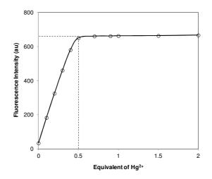
**Fig. S8** Fluorescence intensity changes ( $\lambda_{ex}/\lambda_{em} = 570/594$  nm, slit widths 2.5 nm) of probe **1** (1.0 µM in pure water) as a function of equivalent of Hg<sup>2+</sup> for each addition at room temperature (reacted 15 min and adjusted pH to 7.4 with PBS before determination).
