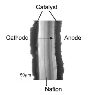
**Figure S1.** Optical image of the Nafion MEA cross-section. The data acquisition direction is indicated by the arrow. The catalyst layers were removed before the in–depth measurements.
