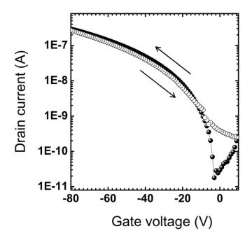
**Figure S3.**  $I_D$ - $V_G$  transfer characteristics of PDHTT-based OTFTs in the saturation regime  $(V_D = -80 \text{ V})$ .
