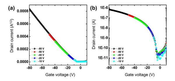
**Figure S4.** (a)  $I_D^{1/2}$ - $V_G$ , (b)  $I_D$ - $V_G$  transfer characteristics of the PDHTT OTFTs at various gate voltages.
