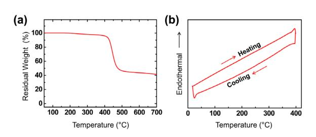
Figure S5. (a) TGA and (b) DSC analyses of PDHTT film.
