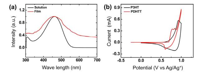
**Figure S2.** (a) UV-Vis absorption spectra and (b) cyclic voltammetry (vs Ag/AgCl) of the PDHTT film.
