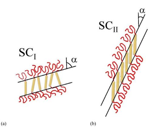
Figure S8. The schematic representations of the  $SC_I$  phase and  $SC_{II}$  phase. (a) Less parallel alignment leads to more space for coil. Small slippage is required and  $SC_I$  phase forms. (b) More parallel alignment results in less space for coil. Large slippage is required and  $SC_{II}$  phase occurs.
