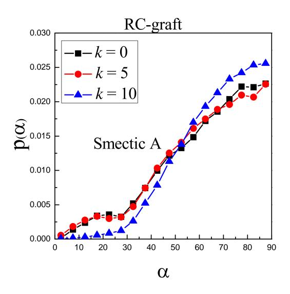
Figure S3. The slippage angle distributions for RC-grafts with varied  $\pi$ - $\pi$  strength(*k*). The rod length =9, coil length = 3, and arm number = 4, respectively.
