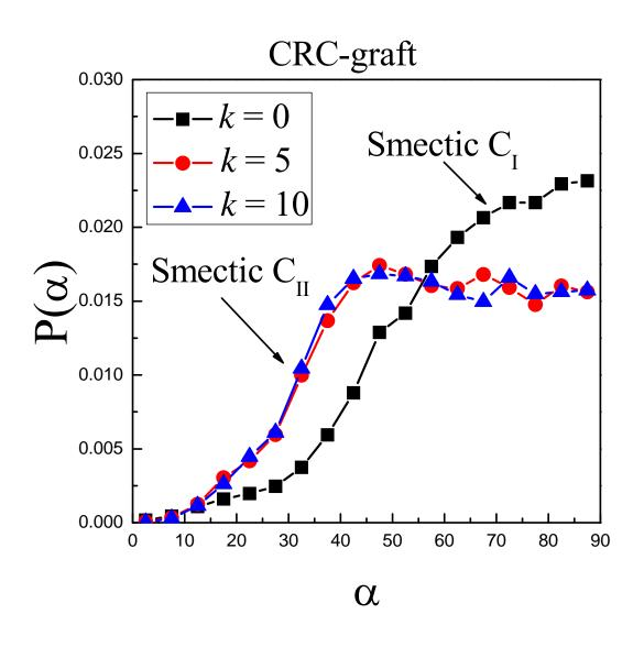
Figure S6. The slippage angle distributions for CRC-grafts with varied  $\pi$ - $\pi$  strength (*k*). The rod length =9, coil length = 3, and arm number = 6, respectively.
