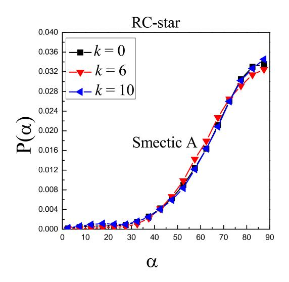
Figure S2. The slippage angle distributions for tri-armed RC-stars with varied  $\pi$ - $\pi$  strength (*k*). The rod and coil lengths are 12 and 4, respectively.
