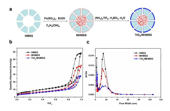
**Figure S1.** a) Schematic illustration of the synthesis strategy of TiO2/MHMSS; b) N2 adsorption-desorption isotherms and c) the pore diameter distributions of HMSS, MHMSS and TiO2/MHMSS materials.
