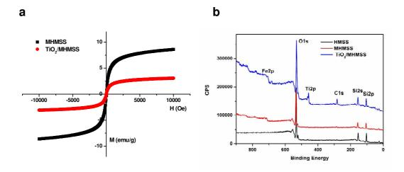
**Figure S2.** a) The magnetization curves of MHMSS and TiO2/MHMSS materials. b) XPS pattern of HMSS, MHMSS and TiO2/MHMSS materials.
