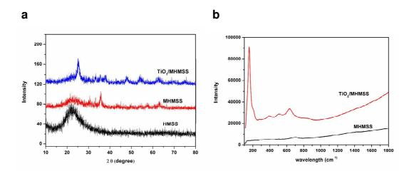
**Figure S3.** a) XRD profiles of HMSS, MHMSS and TiO2/MHMSS materials; b) Raman spectra of MHMSS and TiO2/MHMSS materials.
