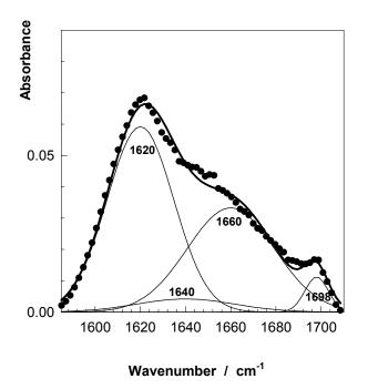
**Figure S3.** Typical ATR-FTIR spectrum of a freeze-dried silk fibroin hydrogel sample formed at pH = 8.3 after baseline correction. The original data are shown by the filled circles while solid curves are the results of curve fitting for the original spectrum (thick curve) and hidden peaks (thin curves).
