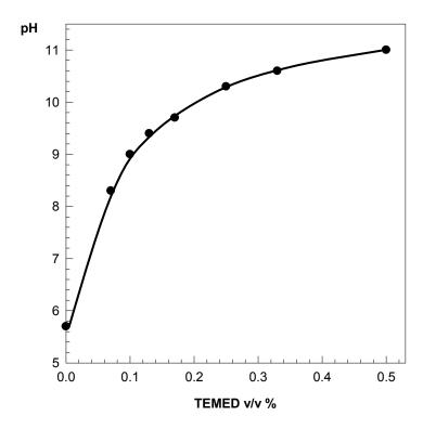
**Figure S1.** pH of the reaction solution shown as a function of TEMED concentration. Silk fibroin = 4.2 w/v %. EGDE = 150 %.
