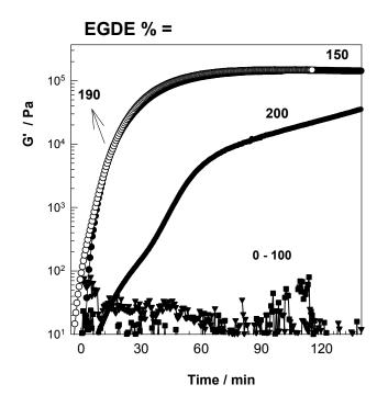
**Figure S4.** Elastic modulus *G' vs* reaction time (except the lag phase) plots during the cross-linking of silk fibroin at 50°C in the presence of various amounts of EGDE indicated. pH = 9.0.  $\omega = 1$  Hz.  $\gamma_0 = 0.01$ .
