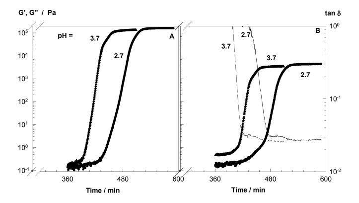
**Figure S5.** *G*' (A), *G*'' (B, symbols) and *tan*  $\delta$  (B, curves) during the cross-linking of silk fibroin at 50°C in the presence of 150 % EGDE. pHs indicated.  $\omega = 1$  Hz.  $\gamma_0 = 0.01$ .
