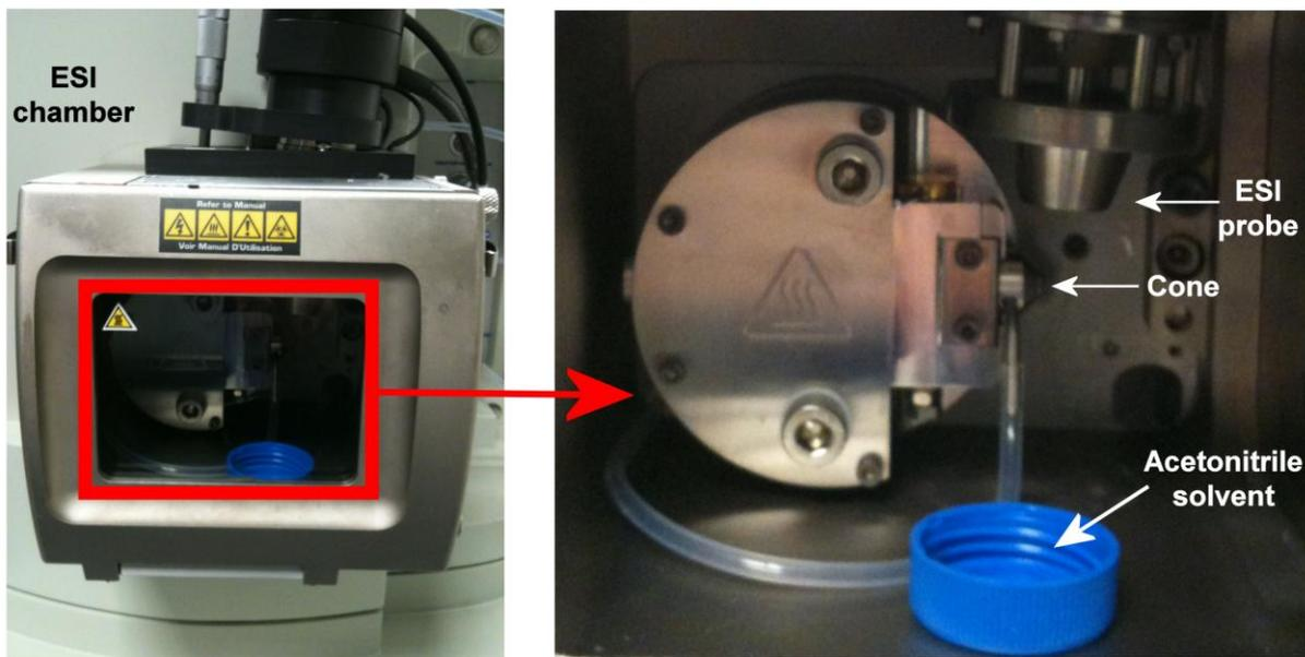
**Figure S1.** Photograph of the acetonitrile solvent container placed inside the doorway of the ESI source chamber.
