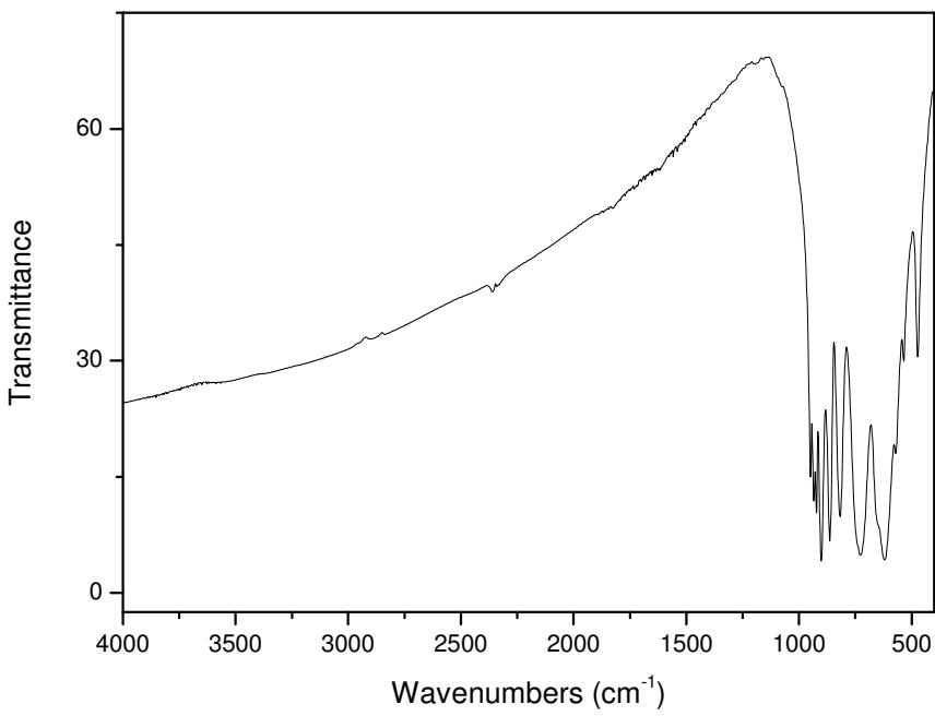
S7. IR spectrum for  $\text{PbMo}_2\text{O}_5(\text{SeO}_3)_2$
