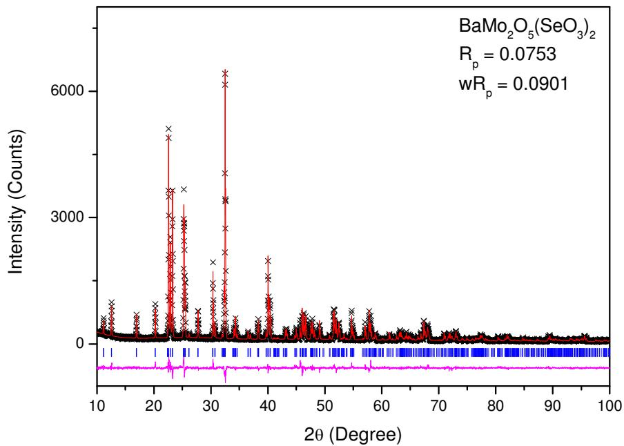
The calculated pattern (red solid line) is compared with observed data ( $\times$ ). The locations of reflections are indicated by the blue vertical bars. The difference between the observed and calculated profiles is shown at the bottom (magenta solid line).
