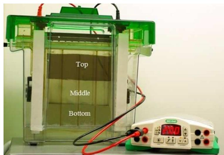
**Figure S1.** Gel electrophoresis apparatus
